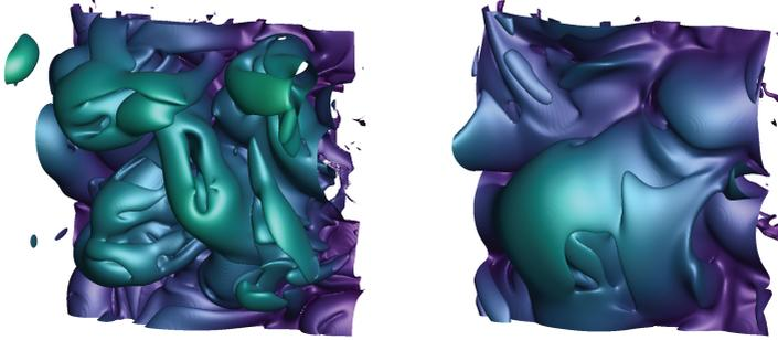
Figure 4.10: Isosurfaces of  $\omega_i^2 = 0.02\omega_{i,b}^2$  for a Newtonian simulation (left) and for a simulation with polymers (right).
