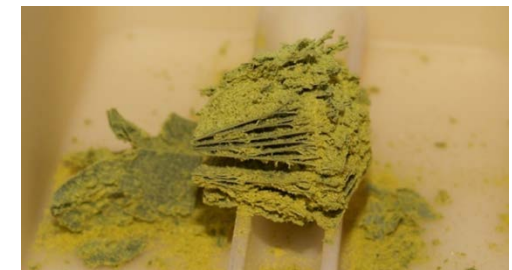
After 48 hours @ 600 °C oxygen atmosphere
