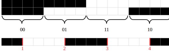
Figure 4: Column extraction process with d = 3 and a resolution of 16 pixels, Gray Code.
