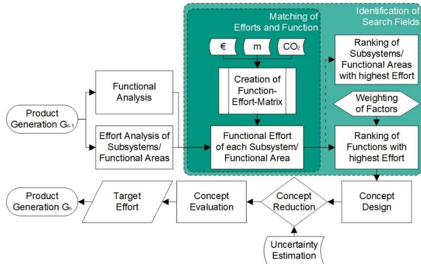
**Fig. 1: Workflow of the Extended Target Weighing Approach**
