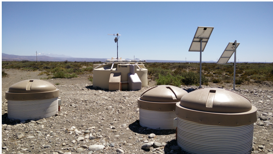
Figure 1.16: A WCD station of the SD-750 is shown a scintillator on top. The capsules in the foreground are access hatches for the surrounding muon counters [68].
