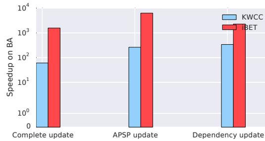
Figure 16: Average speedups on recomputation with BA (geometric mean) over all networks of Table 5, with random weights. The column on the left shows the speedup of the complete update, the one in the middle the speedup of the APSP update only and the one on the right the speedup of the dependency update only.
