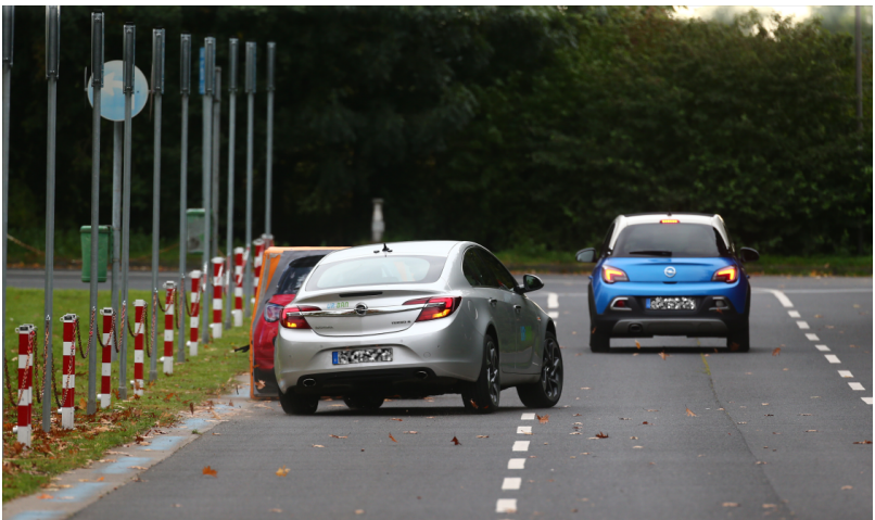
Figure 6.1: Automated collision avoidance maneuver performed in a test vehicle
