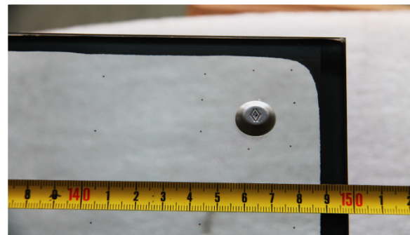
Figure 1: Evacuation vent and distance pillars in a vacuum glass (from the company Synergy/picture credit: Holzforschung Austria).
