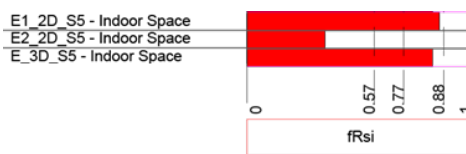
Figure 4: Simulation results of a vacuum glass pane: f_{Rsi} -values (E1 – 2D simulation without pillars, E2 – 2D simulation with pillars, E – 3D – simulation) (Pont and Mahdavi 2017)
