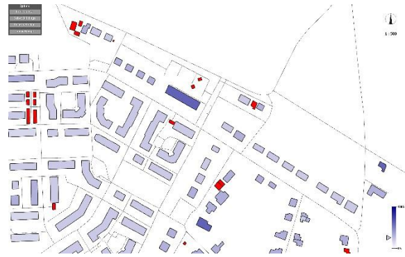
Figure 5: Representation of the percentage of electricity consumption that can be covered by solar energy; buildings marked in red are excluded from the analysis.
