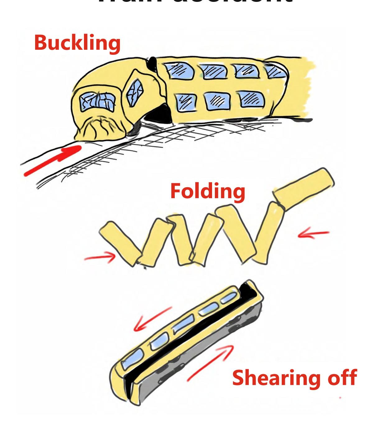
**Summary:** In our opinion, accidental damage is greater if the individual shells are omitted, meaning communitarization of the interior and release of relative movements between vehicle and passengers.
