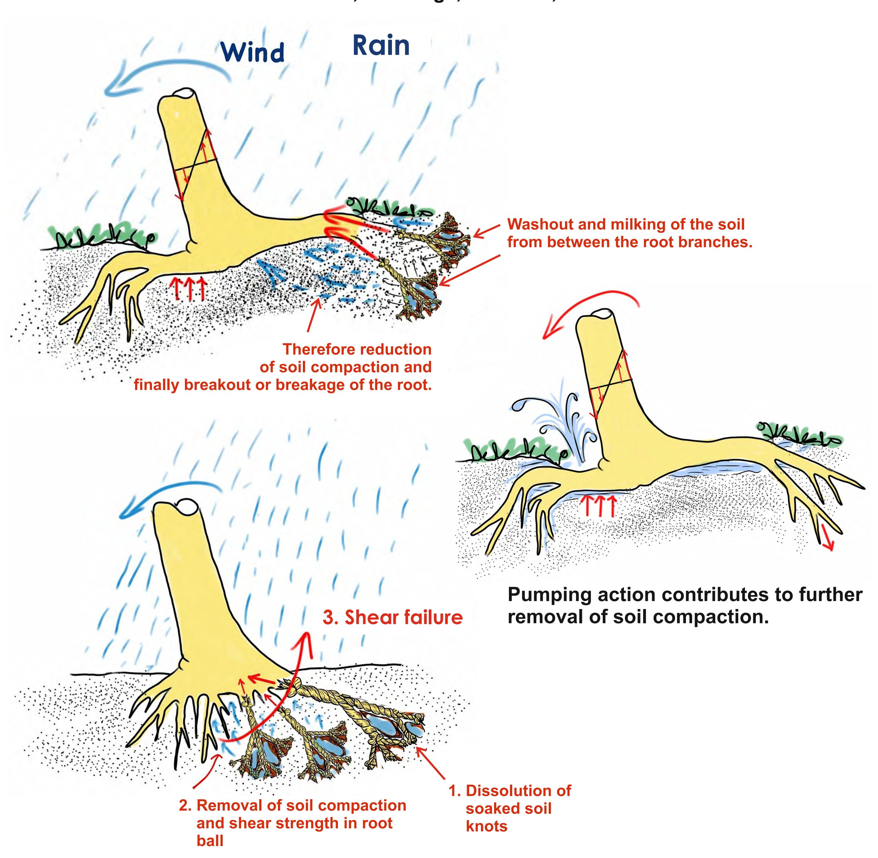
**Summary:** For both types of anchors, the failure starts with resolution and milking the soil from the root branches. This will decrease soil compaction and result in a pull out of the horizontal root or shear failure of the root ball.
