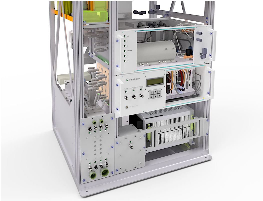
Figure 3.23.: CAD drawing of the new PTRMS-CARIBIC installed in the instrument rack. Please note that the picture is not complete. Some parts and accessories are missing to give a better insight. In contrast to the hitherto used PTRMS, the new device saves so much space and weight that a further instrument can be installed in the rack. Image courtesy of Simon Heger (KIT).
