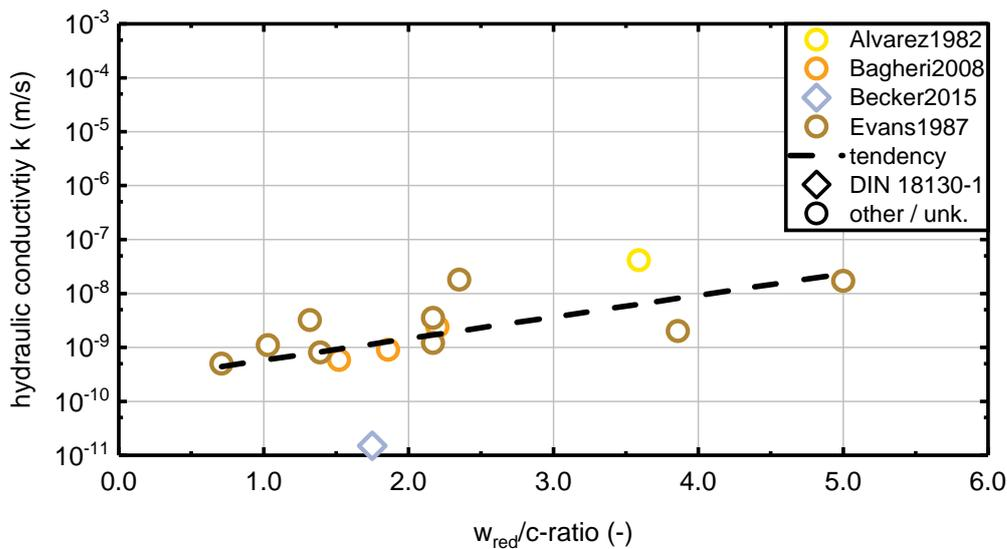
Figure 4.1: Hydraulic conductivity of Plastic Concrete over  $w_{red}/c$ -ratio at  $\sigma_c = 0$
