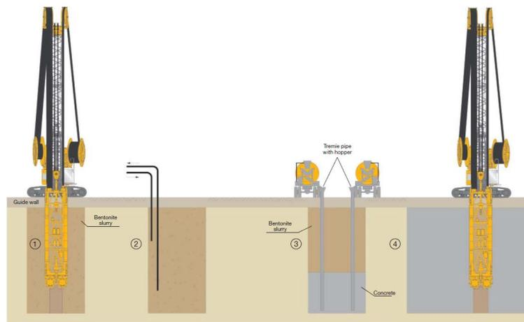
Figure 1.2: Construction of a Cut-Off Wall with the Two-Phase Method [27]
