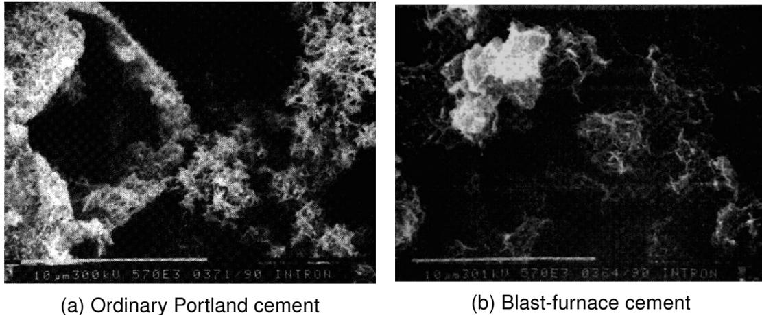
Figure 2.1: SEM images of the micro-structure of hardened cement-bentonite mixtures depending on cement type used [55]
