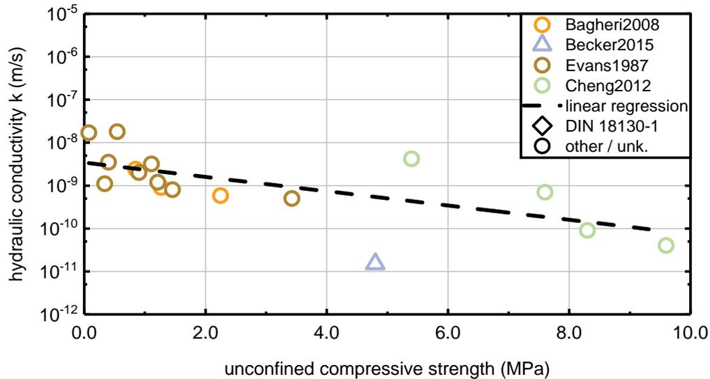
Figure 4.2: Hydraulic conductivity of Plastic Concrete over compressive strength
