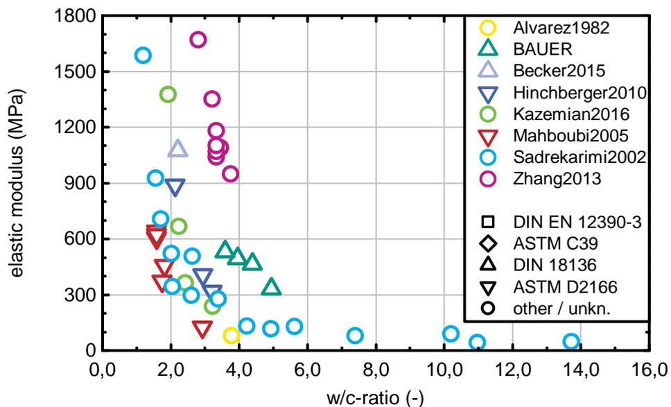
Figure 3.7: Overview of the elastic modulus as a function of the w/c-ratio at 28 days
