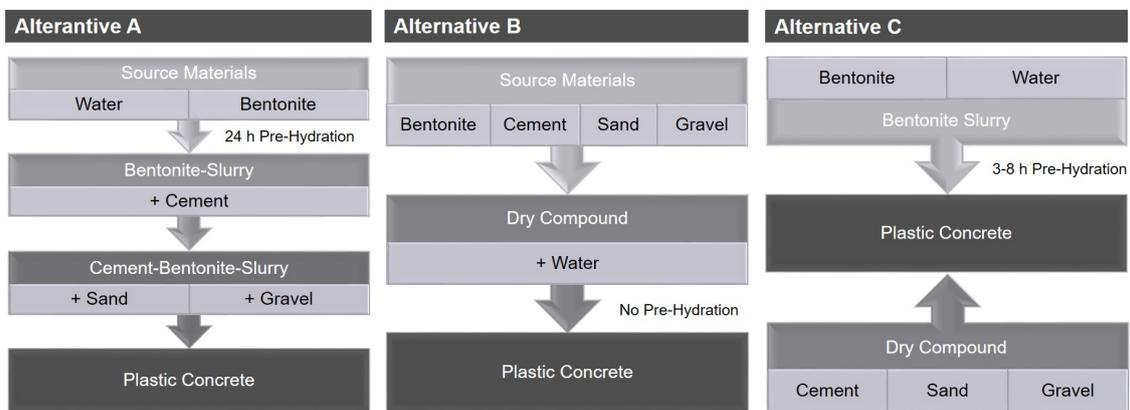
Figure 2.5: Representative examples of Plastic Concrete mixing sequences
