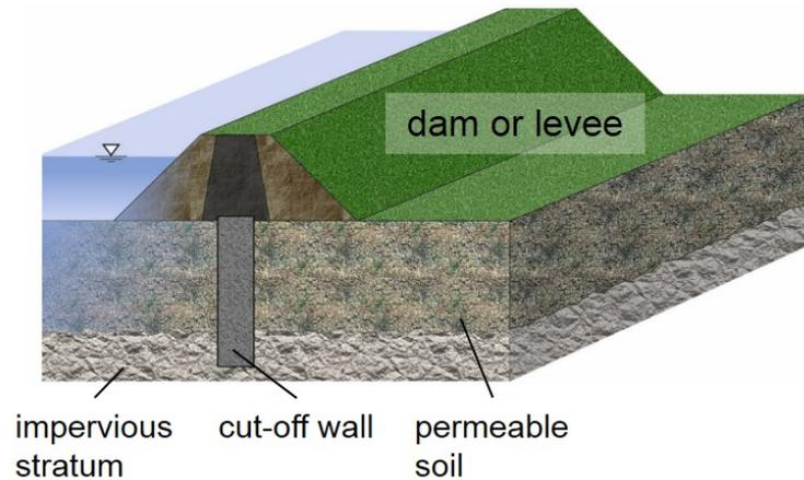
Figure 1.1: Schematic of an Earth Dam with Cut-Off Wall
