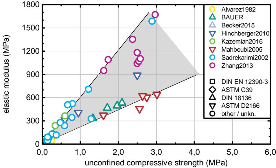
Figure 3.8: Elastic modulus as a function of the compressive strength at 28 days
