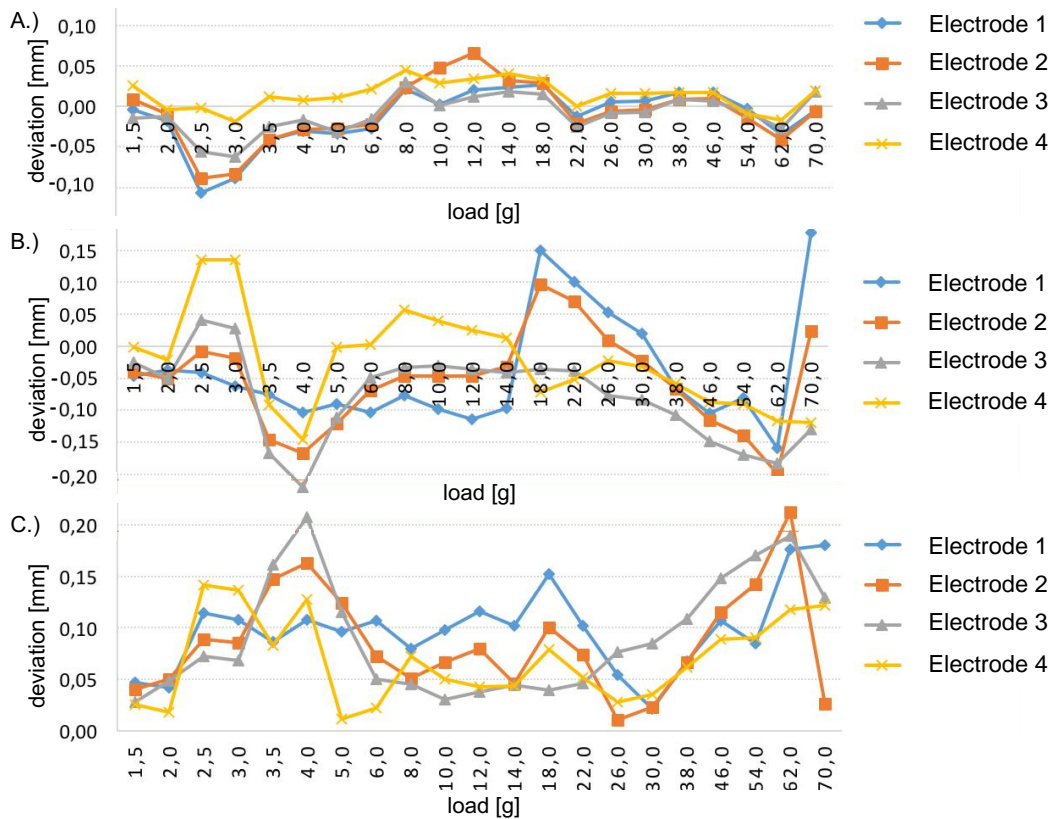
Figure 5.10: Deviation of (A) x electrode coordinates, (B) y electrode coordinates and (C) z electrode coordinates in the first spline dependent on the force at the E-module of 621.5 MPa. The figure is adapted from [S9], [152].
