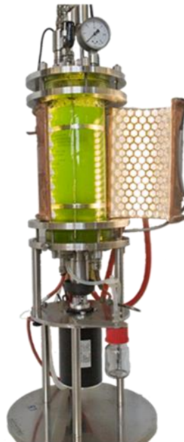
Figure 11-3. 1.8L model reactor. KLF 2000 bioreactor (Bioengineering AG).
