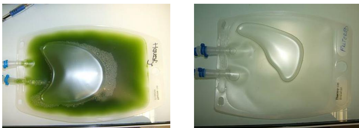
Figure 8-6. Concentrated algae suspension (left side) and cell-free medium (on the right) after passage through the integrated harvesting unit during the second flight operating as chemostat. (Podhajsky 2014)
