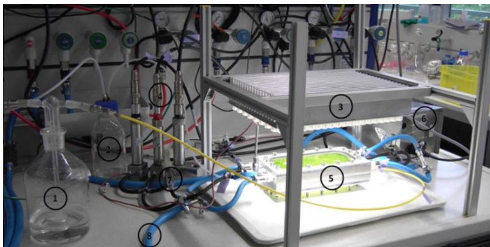
Figure 3-4. Setup of membrane-aerated photobioreactor with periphery in batch mode. (1) Inlet air water vapor saturation bottle, (2) capture bottle for condensate, (3) warm-white LED panel, (4) probes for DO, d\text{CO}_2 , pH, p, T, (5) photobioreactor with membrane(s), (6) pump, (7) sampling via safelock, (8) cooling water circuit. Optionally exhaust gas is connected to GC for analysis of \text{CO}_2 , \text{O}_2 and \text{N}_2 .
