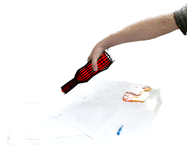
(b) 3D point cloud with segmented bottle.
