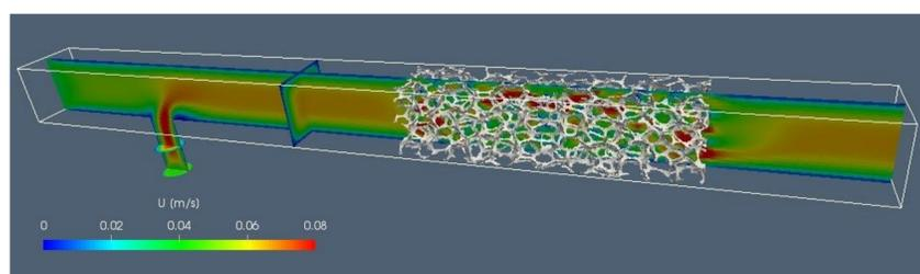
Fig. 3: Steady velocity field of single phase flow simulation with liquid entering at both inlets.
