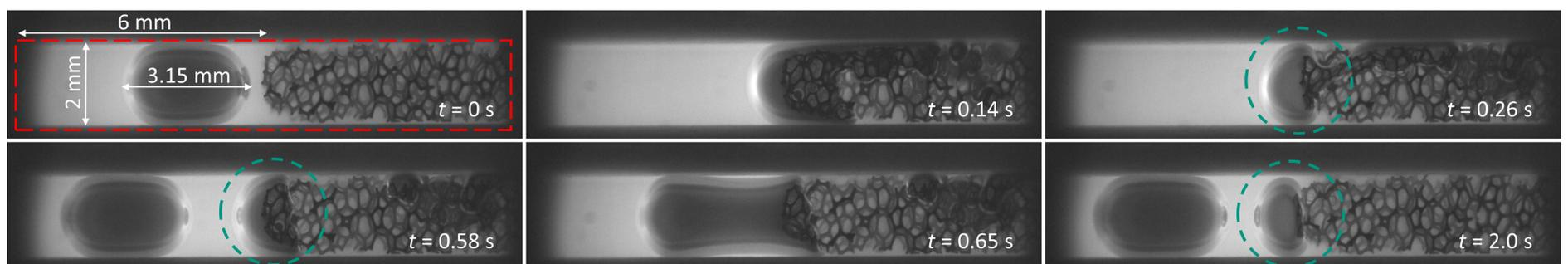
Fig. 2: Visualizations of the penetration of individual Taylor bubbles into the porous medium at six instants in time. The top row shows the same bubble.
