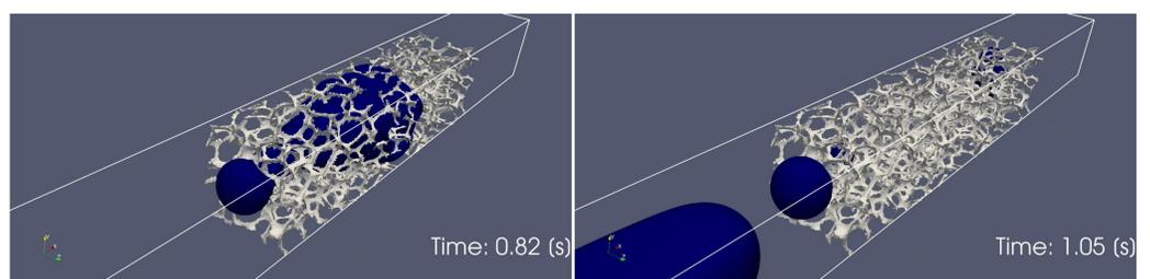
Fig. 4: Pinch-off of first Taylor bubble (left) and approach of the 2<sup>nd</sup> Taylor bubble (right). Similar to the experiment, gas is captured in front of the foam. A similar simulation with surface tension reduced by 50% shows penetration of the entire Taylor bubble instead.
