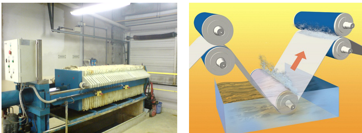
Figure 6.10: Potential setups that could serve as a model for a continuous process: Filter chamber press (left) and roll to roll process (right). Figures are taken from [Murúg07, Limited13].
