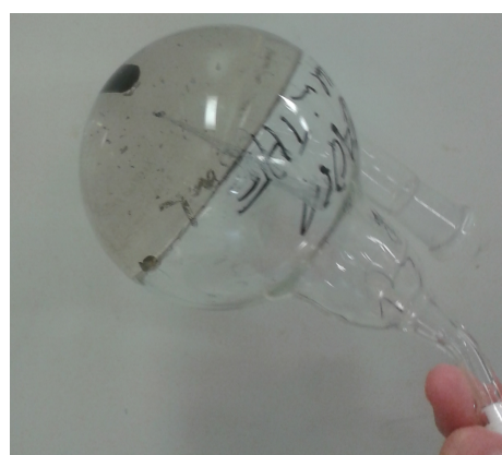
Figure 4.16: End-linking of living Pt BMA polymer chains by the addition of EGDMA in the anionic polymerization. Left) Use of a monofunctional initiator results in the formation of a narrow distributed 5-arm star polymer, as shown in the SEC elugram. Right) Use of a difunctional initiator yields a transparent organogel.
