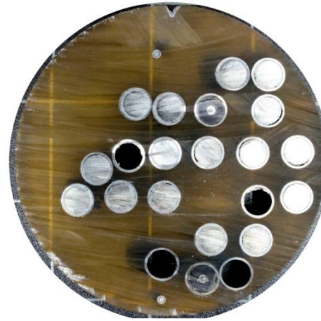
1480 mm: intact rods, slightly oxidized clads
