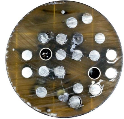
1430 mm (upper spacer grid): loss of clads
