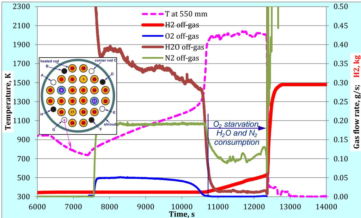
Fig. 6. Outlet gas behaviour during air ingress: gas consumption phenomena.
