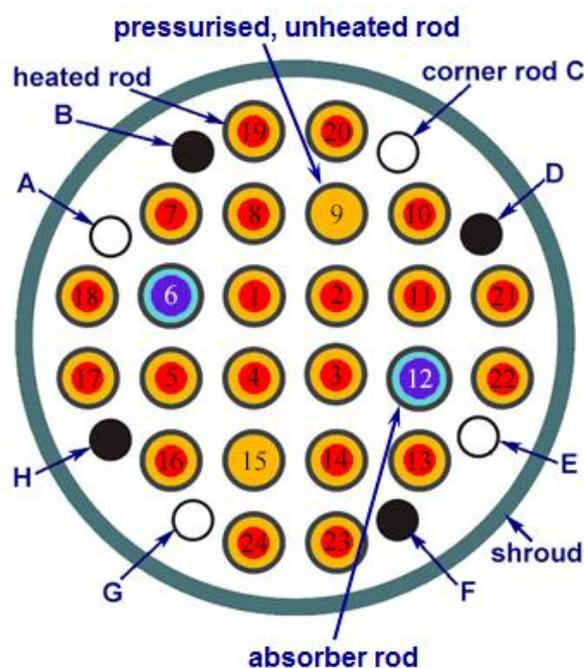
Fig. 2 QUENCH-18 Bundle Cross Section.
