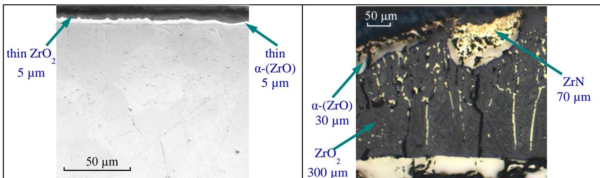
Fig. 7. Comparison of corner rod structures at elevation of about 520  $\mu\text{m}$  for rod D withdrawn at the air ingress initiation (left side) and rod H withdrawn at the end of temperature escalation (right side).
