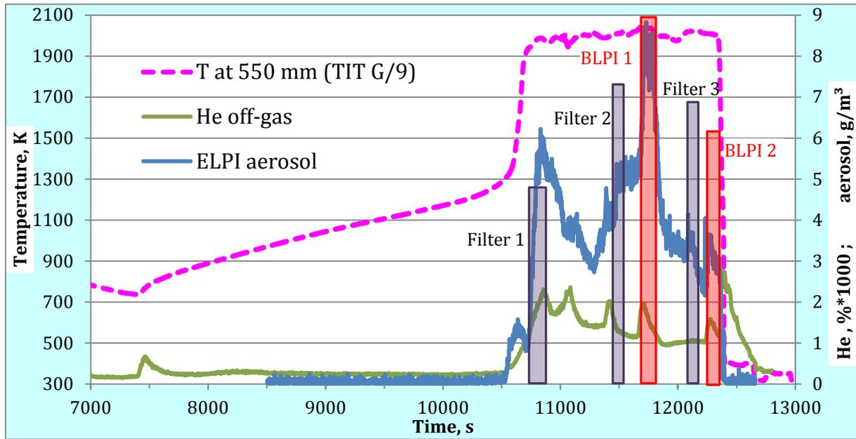
Fig. 5. Failure of absorber rods with aerosol release.
