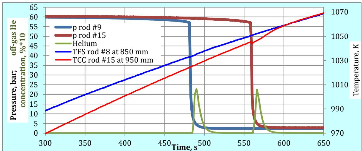
Fig. 4. Burst of pressurised rods #9 (at  $\approx 850$  mm) and #15 (at 950 mm).
