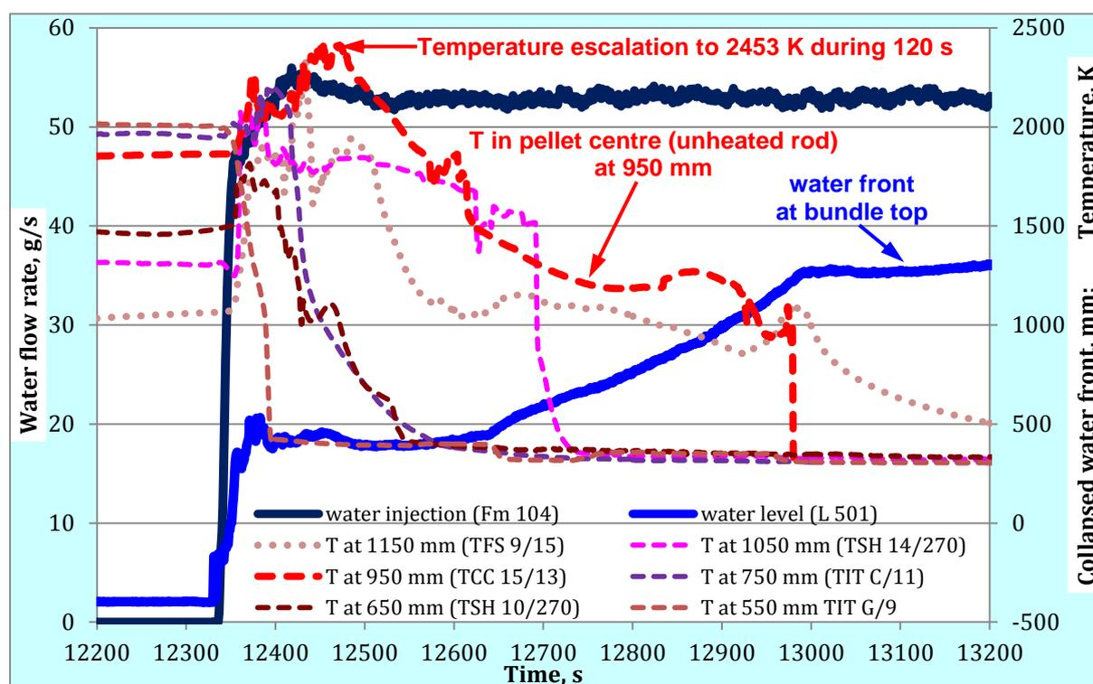
Fig. 8. Progress of collapsed water front and temperatures during the reflood phase.
