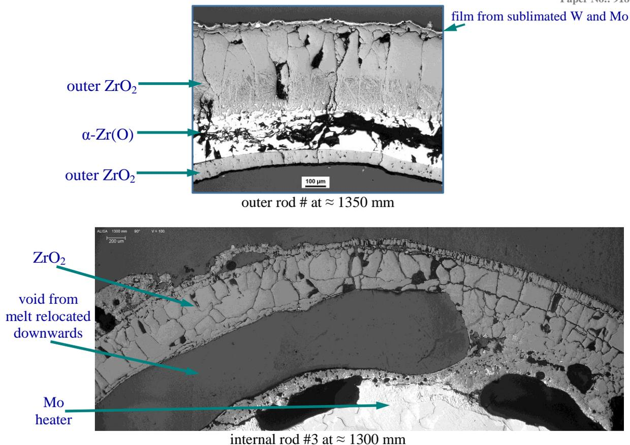
Fig. 10. Cladding structures of outer and internal rods at upper bundle elevations.
