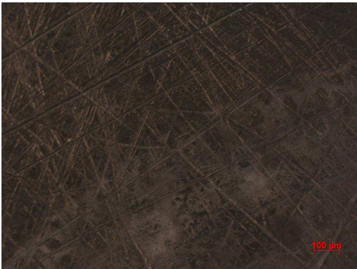
Figure 4.3. – Optical image of the surface for the polished tungsten foil as working electrode before the deposition of aluminium.
