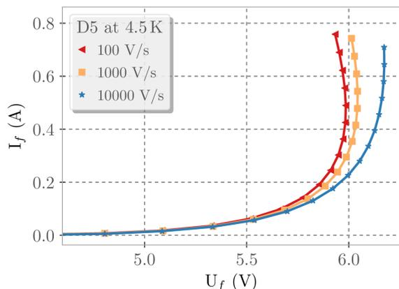
Figure 3: Turn-on voltage measured on D5 (N-base width -10 μm) for different voltage ramp rates at 4.5 K.
