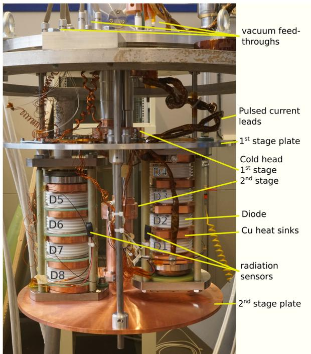
Figure 2: Picture of the cryostat setup demonstrating the assembly and placement of the diodes.
