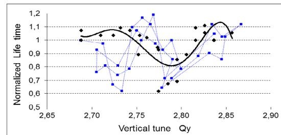
Figure 4: Normalized lifetime as a function of the vertical tune. Black dots and fit by a polynomial (black curve) are for the case that CATACT is OFF. The dip in lifetime at  $Q_y = 2.78$  is seen during the crossing of the structure resonance  $Q_x - Q_y = 4$ . The blue dots for  $B_{CAT} = 2.5 \text{ T}$  show an additional drop in the lifetime at  $Q_y = 2.724$  ( $Q_x = 6.776$ ), corresponding to the coupling octupole resonance  $2Q_x + 2Q_y = 19$ .
