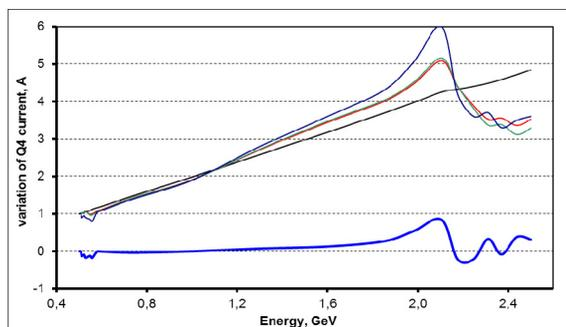
Figure 6: Corrections to ramp table to stabilize vertical tune during energy ramp from 0.5 to 2.5 GeV. Black curve - proportional increase of quads current during ramp. Blue, green and red curves around black curve - deviation of quad current from linear fit in order to minimize tune shaking. Blue line at bottom - difference between simulations and experimental tests.
