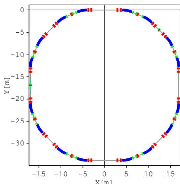
Figure 1: Model of the KARA ring [2]. The  $22.5^\circ$  bending magnets are depicted in blue, quadrupoles in red and the sextupoles are marked in green. The CATACT/CLIC wigglers are shown by long green strips. Octupole components of wigglers are represented by brown strips in the middle of insertion device.
