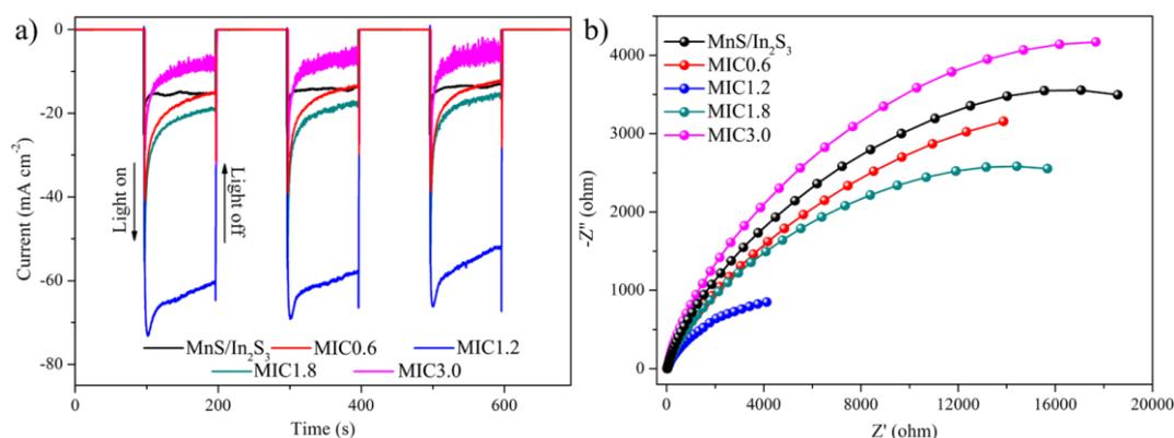
**Fig. 3.** a) Transient photocurrent response, b) EIS of all the prepared samples. Test conditions: The photoelectrochemical measurements over all the samples at open circuit potential were tested under visible-light irradiation ( $\lambda > 420$  nm), the 1.2 M Na<sub>2</sub>SO<sub>3</sub> solution as electrolyte.
