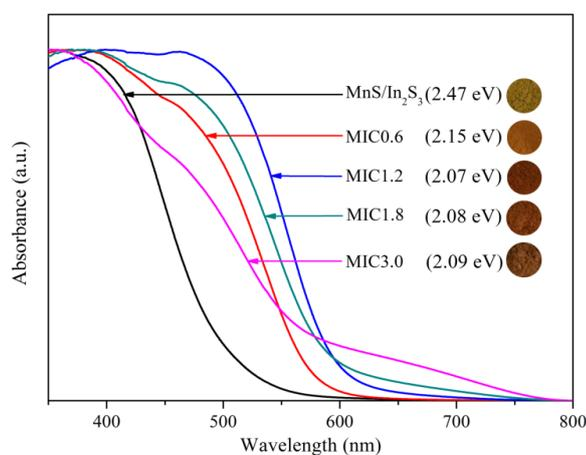
**Fig. 2.** UV-vis DRS of the prepared samples.
