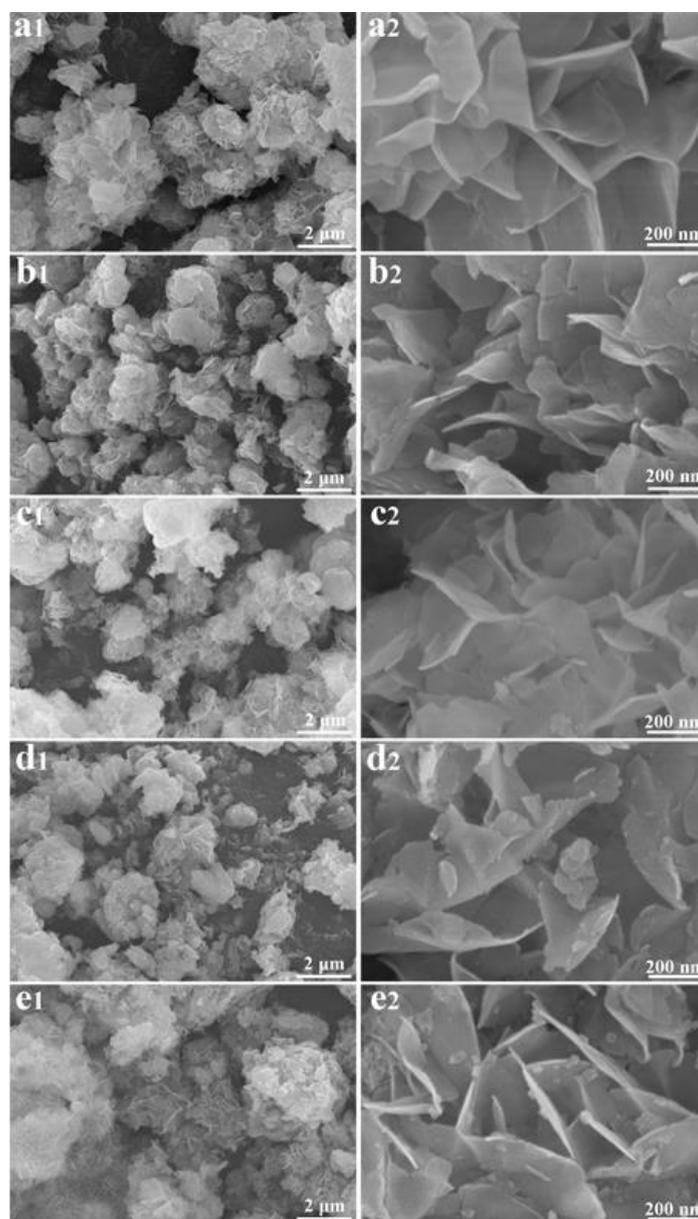
**Fig. 6.** SEM images of MIC samples: a1) Low- and a2) high-magnification SEM images of sample MnS/In<sub>2</sub>S<sub>3</sub>; b1) Low- and b2) high -magnification SEM images of MIC0.6; c1) Low- and c2) high -magnification SEM images of MIC1.2; d1) Low- and d2) high -magnification SEM images of MIC1.8; (e1) Low- and e2) high -magnification SEM images MIC3.0.
