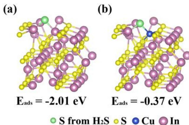
**Fig. 8.** The structures of S adsorbed on the surface of (a)  $\beta-In_2S_3$  and (b)  $Cu-In_2S_3$ .
