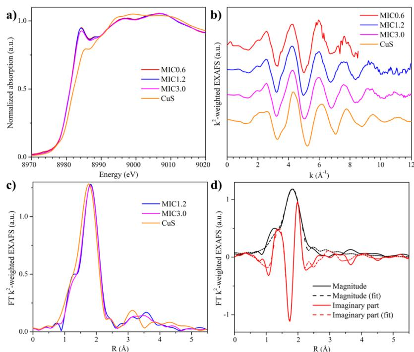
**Fig. 5.** a) XANES, b)  $k^2$ -weighted EXAFS, and c) Fourier-transformed (FT)  $k^2$ -weighted EXAFS spectra (in the  $k$ -range 2.3-10.7 Å<sup>-1</sup>, uncorrected for the phase shift) of the  $\text{MnS}/(\text{In}_x\text{Cu}_{1-x})_2\text{S}_3$  composites with the CuS reference spectrum; d) fit of the EXAFS spectrum of the MIC1.2 sample.
