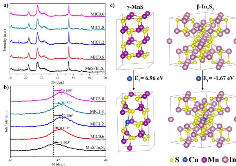
**Fig. 4.** a, b) XRD patterns of all the samples, c) The crystal structures of MnS and In<sub>2</sub>S<sub>3</sub> before and after the introduction of Cu.
