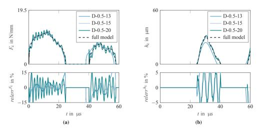
**Figure 4.12:** Results of the damping approach for various numbers of dynamically considered modes  $n_{dc}$  and a fixed damping ratio of  $\zeta = 0.5$ . The upper plots show the central force  $F_c$  (a) and central gap height  $h_c$  (b) over time t and the lower plots show the respective relative deviation of the reduced order model from the full model relerr  $F_c$  (a) and relerr  $h_c$  (b) over time t.
