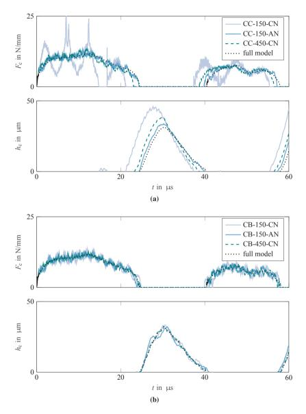
**Figure 4.10:** Central force  $F_c$  (upper subfigure) and central gap height  $h_c$  (lower subfigure) over time t. The results are computed with Craig-Chang method based reduced order models (a) and Craig-Bampton method based reduced order models (b). The results of the full model are plotted for comparison. The characteristics of the reduced order models are summarized in Tab. 4.4.
