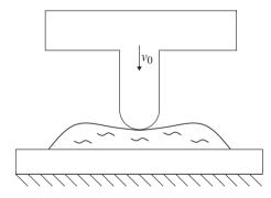
**Figure 4.23:** Exemplary drawing of the impact of the axisymmetric T-geometry on a lubricated plate. The T-geometry moves with initial velocity  $v_0 = 0.313$  m/s from the initial height  $h_0 = 30$  µm towards the plate.
