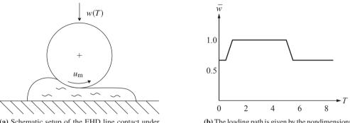
(a) Schematic setup of the EHD line contact under combined entraining and squeeze motion.
