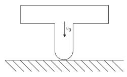
**Figure 4.8:** Schematic of the example problem setup. The elastic T-geometry moves with the initial velocity  $v_0$  towards the rigid plate. It impacts the plate and rebounds from it. After the rebound it impacts the plate again because of the geometrical shape of the body and its elastic deformation.
