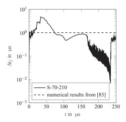
**Figure 4.22:** Time step size  $\Delta t_j$  of the current model (S-70-210) and of [85]. During the early impact phase, a large step size  $\Delta t_j$  is sufficient to approximate the pressure build up and motion of the sphere. During the rebound phase, pressure peaks move through the contact, see Fig. 4.19, and the step size is reduced significantly to capture these. After the rebound (at around 236 µm), the sphere flies freely and the step size increases rapidly.
