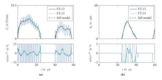
**Figure 4.14:** Results of the feedthrough approach. The upper plots show the central force  $F_c$  (a) and central gap height  $h_c$  (b) over time *t*. The lower plots show the respective relative deviation of the reduced order model from the full model *relerr*  $F_c$  (a) and *relerr*  $h_c$  (b) over time *t*.
