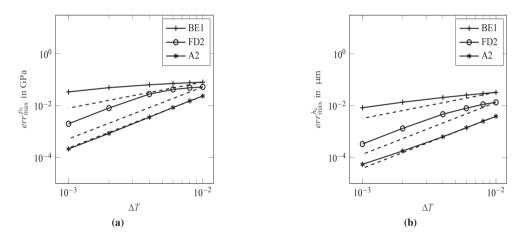
Figure 4.5: Order investigation for the central pressure  $p_c$  (a) and for the central gap height  $h_c$  (b). The slope of the dashed line indicates the theoretical convergence order of the respective method.
