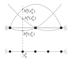
**Figure 3.2:** Quadratic shape functions of a one-dimensional structure element, which consists of three structure nodes. The shape functions are evaluated at the fluid node  $x_{i_F}^F$ . The values of the shape functions at the fluid node give the weights for the interpolation matrix  $G_{SF}$ , see Eq. (3.29).
