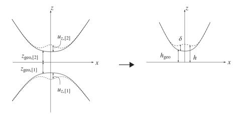
**Figure 2.1:** The displacements of the lower and upper body, i.e.,  $u_{z,[1]}$  and  $u_{z,[2]}$ , are combined via Eq. (2.43) to give the gap displacement  $\delta$ . Analogously, the undeformed geometries of the lower and upper bodies, i.e.,  $z_{geo,[1]}$  and  $z_{geo,[2]}$ , are combined to give the undeformed gap height  $h_{geo}$  using Eq. (2.44). The sum of both quantities gives the deformed gap height h.
