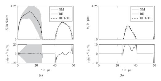
**Figure 4.16:** Results of the example problem with different time integration methods: Backward Euler method (BE1), the Newmark  $\beta$ -method (NM) and the Hilber-Hughes-Taylor method (HHT-TF). The upper plots show the central force  $F_c$  (a) and central gap height  $h_c$  (b) over time t. The lower plots show the respective relative deviation of the reduced order model from the reference solution relerr  $F_c$  (a) and relerr  $h_c$  (b) over time t.
