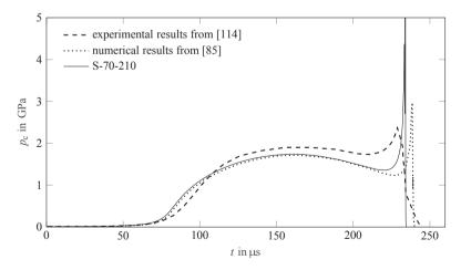
**Figure 4.21:** Central pressure  $p_c$  over time *t*. The results of the developed extended EHD contact model (S-70-210, see Tab. 4.7) are compared with numerical results [85] and experimental results [114].
