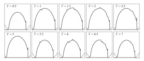
Figure 4.2: The plots show the pressure (thick line) and the gap height (thin line) spatially resolved at different time instances. The upper row shows the loading phase and the lower row shows the unloading phase.
