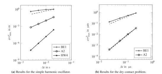
Figure 4.17: For each time step size and time integration method the deviation  $err_{max}$  of the computed results from the reference solution is plotted over the step size  $\Delta t$ . The slope of the dashed line indicates the theoretical convergence order of the respective method.
