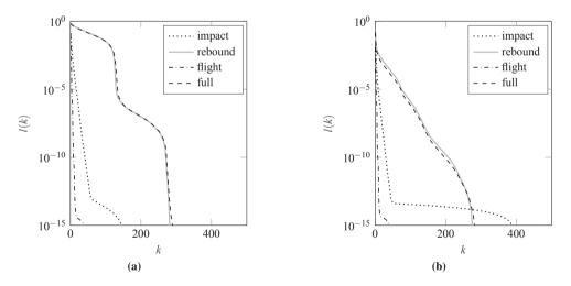
**Figure 4.28:** Loss value l(k) over system size k for the pressure (a) and for the gap height (b). The different decay rate of the loss value in the different phases indicates the difference in the similarity of the solutions in the different phases. A steeper decay typically results in a smaller system size.
