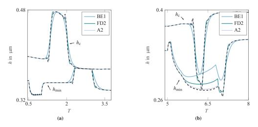
**Figure 4.4:** Central gap height  $h_c$  and minimum gap height  $h_{min}$  during the loading phase (a) and unloading phase (b) over nondimensional time *T*. The results are computed using Backward Euler method (BE1), second-order finite difference method (FD2) and Alexander's second-order method (A2) with the nondimensional step size  $\Delta T = 0.01$ . The dashed line is the reference solution. It is computed using FD2 with  $\Delta T = 1 \cdot 10^{-4}$ .
