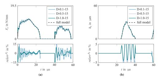
**Figure 4.13:** Results of the damping approach for various damping ratios  $\zeta$  and  $n_{dc} = 15$ . The upper plots show the central force  $F_c$  (a) and central gap height  $h_c$  (b) over time t. The lower plots show the respective relative deviation of the reduced order model from the full model relerr  $F_c$  (a) and relerr  $h_c$  (b) over time t.
