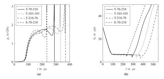
**Figure 4.24:** Central pressure  $p_c$  (a) and central gap height  $h_c$  (b) over time *t*. Table 4.7 lists the elastic material properties of the four setups.
