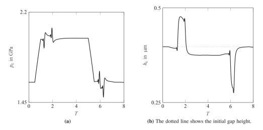
**Figure 4.3:** Central pressure  $p_c$  (a) and central gap height  $h_c$  (b) over nondimensional time *T*. The changes in the pressure and the gap height shortly after the load change are particularly visible in this representation.
