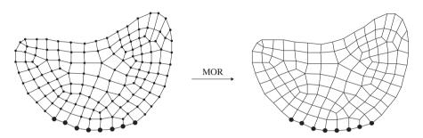
**Figure 2.2:** Model order reduction (MOR) techniques aim to express the behavior of a high-dimensional model (left) by a reduced order model (right). The reduced order model shall consist of a much lower number of degrees of freedom. This is exemplarily shown for a structural finite element model, where only the behavior of the highlighted nodes is of interest. Hence, the MOR procedure aims to express the behavior in this region with as few degrees of freedom as possible.
