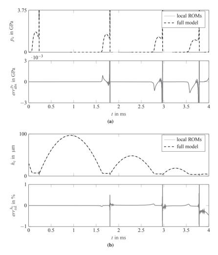
**Figure 4.29:** The upper plots show the central pressure  $p_c$  (a) and central gap height  $h_c$  (b) over the time *t*. The lower plots show the respective absolute deviation of the reduced order model from the full model  $err_{abs}^{p_c}$  (a) and  $err_{abs}^{h_c}$  (b) over the time *t*.
