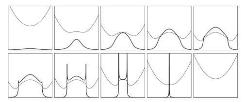
Figure 4.19: Temporal evolution of the pressure (thick line) and the gap height (thin line) spatially resolved in the contact region. The upper row shows the impact phase and the lower row shows the rebound phase.
