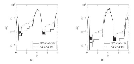
**Figure 4.6:** Time step size  $\Delta T_j$  over time *T* for desired approximate relative deviation of  $relerr_{\max}^{P_c} \approx 3\%$  (a) and  $relerr_{\max}^{P_c} \approx 1\%$  (b). Table 4.2 summarizes the characteristics of the different cases.
