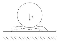
**Figure 4.18:** Schematic of the axisymmetric lubricated impact problem. The sphere moves with initial velocity  $v_0 = 0.313$  m/s from the initial height  $h_0 = 30 \,\mu\text{m}$  towards the plate.
