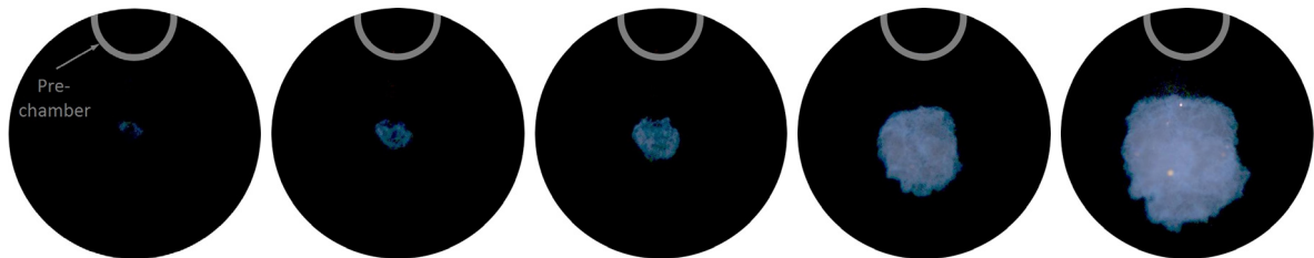
(a) t=6.40 ms (b) t=6.56 ms (c) t=6.72 ms (d) t=7.20 ms (e) t=7.68 ms Figure 8: ignition and combustion process in main chamber of double stage mode ( 1 \times \Phi 1.6 mm case, 1.4 MPa at spark timing, contrast improved)
