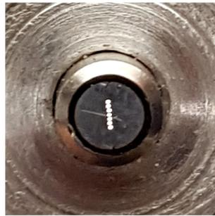
Figure 2: Linear bundle end of the fiber-optic cable.
