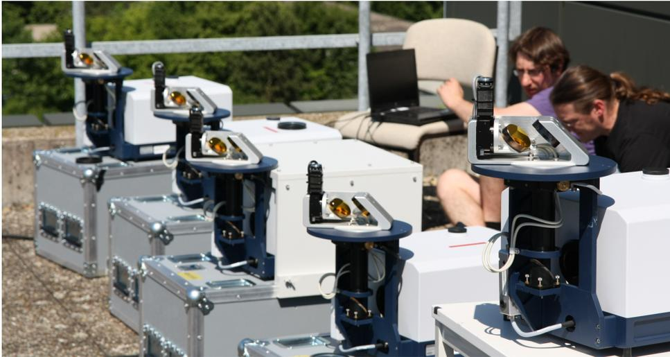
**Figure 4.10:** Calibration measurements performed prior to a campaign on top of the KIT - IMK office building North of Karlsruhe. The instrument in the middle shows a sun cover. Photograph courtesy of F. Hase.
