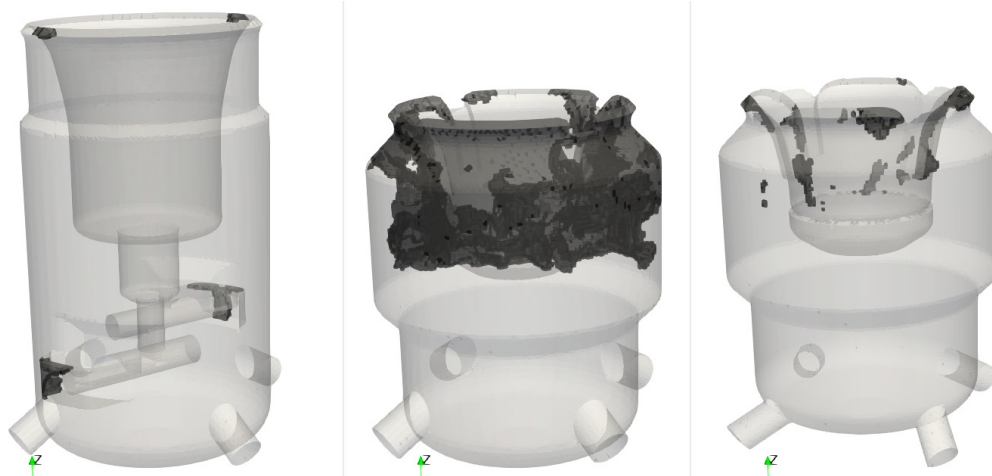
Figure 10: Residual gas distribution in a cut through the symmetry plane at 20°bTDC for 1500 rpm showing only region with a residual gas fraction higher than 20%.
