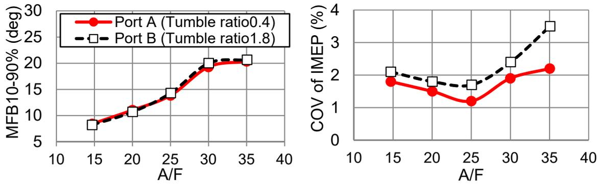
Figure 16: Performance result of Intake ports with different tumble ratios
