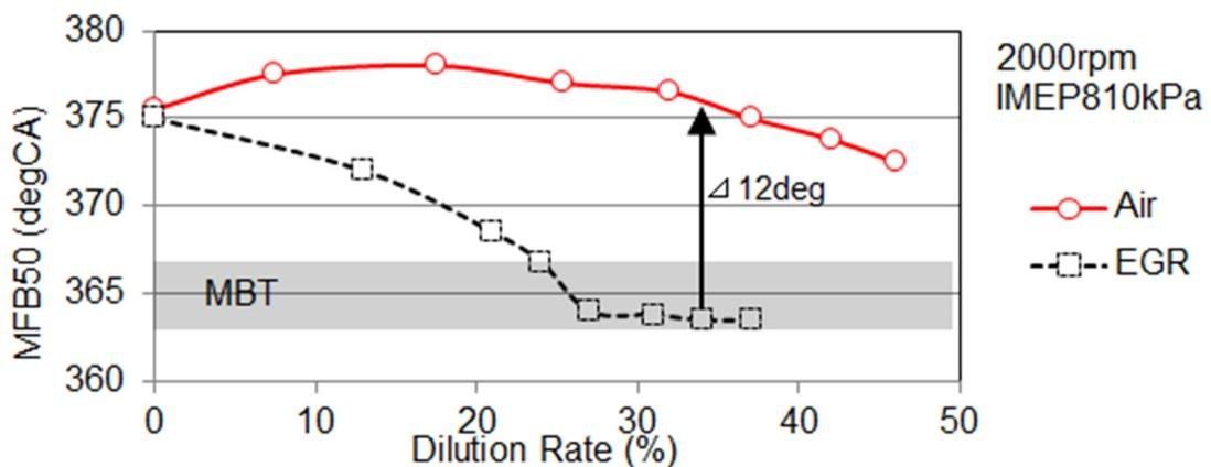
Figure 2: Effect of dilution rate to MFB 50% characteristics
