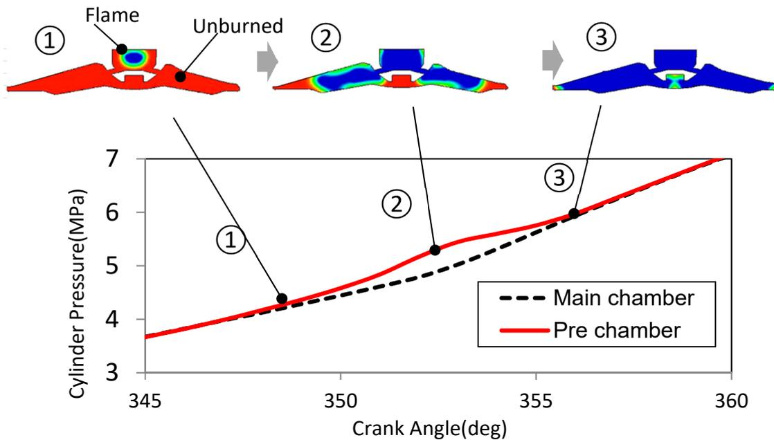
Figure 5: Pre-chamber combustion process at 2000rpm IMEP810kPa
