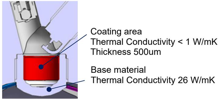
Figure 13: Thermal insulation coating area of pre-chamber
