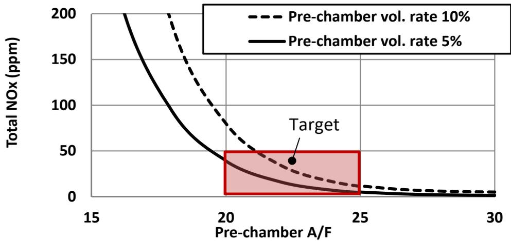
Figure 7: Relation of pre-chamber A/F, Vol and NO<sub>x</sub>
