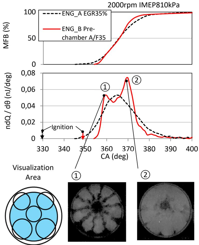
Figure 12: Combustion characteristics and flame visualization of Pre-chamber combustion
