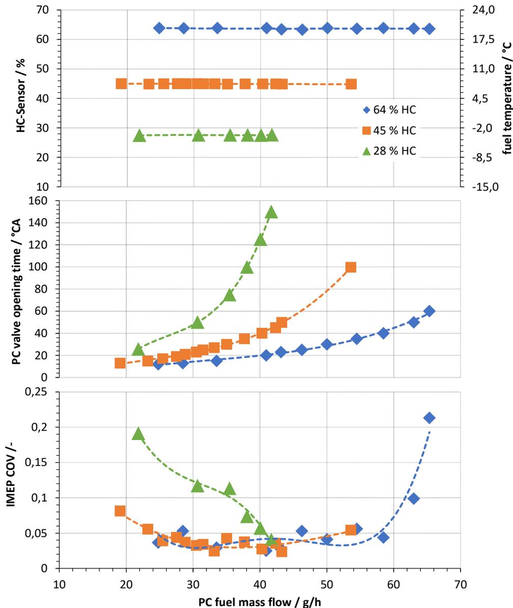
Figure 8: Variation of PC fuel mass flow for different HC-concentrations with VK 3 at  $\lambda = 1.65$ , 4.5 bar IMEP and 1500 rpm
