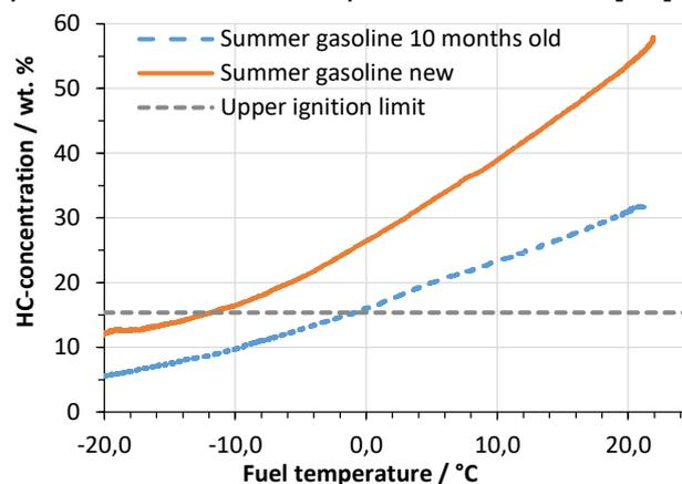
*Figure 1: HC-concentration in the vapour versus fuel temperature*
