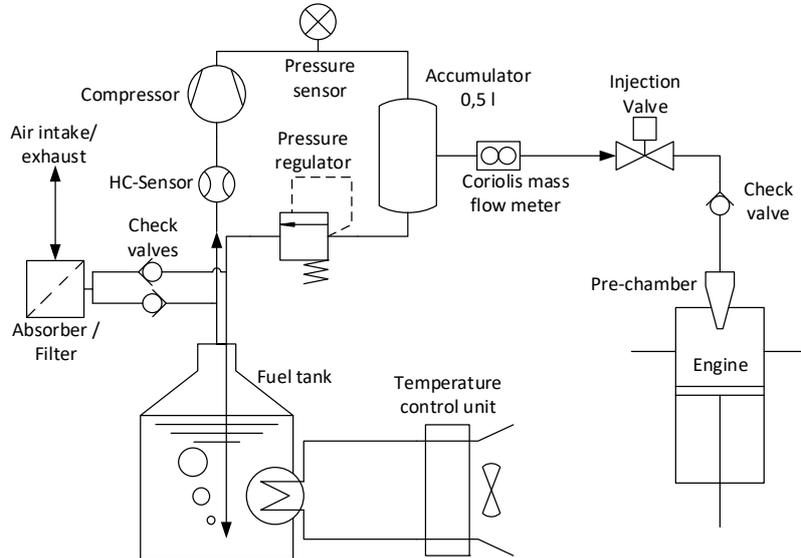
Figure 2: flow chart of the pre-chamber fuelling system
