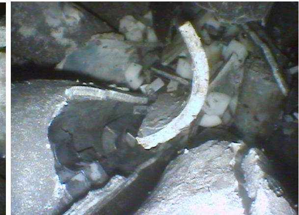
1100 mm: view of oxidized Zry claddings after partial removal of debris
