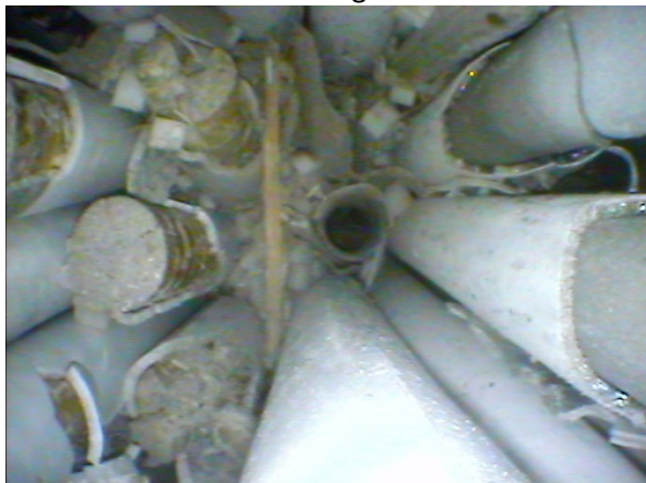
1180 mm after strong mechanical intervention (shaking): spalling of oxide layers and emptying of rod #6
