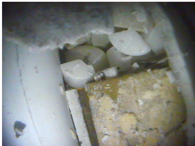
920 mm: relocated pellet segments pellet segment stack of rod #7
