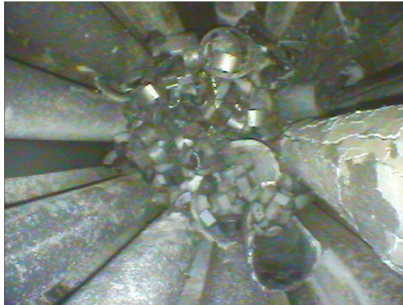
1150 mm: pellet segments inside Zry claddings and at the top of GS #3; through going cracks inside strong oxidized cladding #8; intact oxide of Hf claddings
