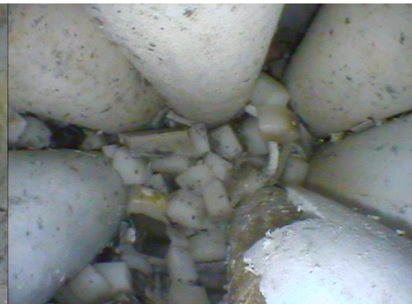
910 mm: view through rod #6, blockage of cooling channel
