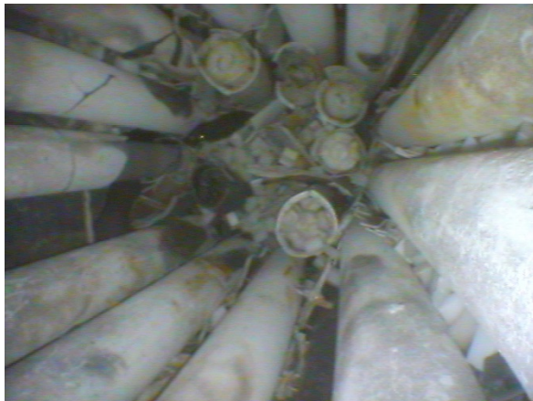
1180 mm: overview of broken central rods with Zry claddings and almost intact (partial \text{HfO}_2 spalling) peripheral heated rods with Hf claddings
