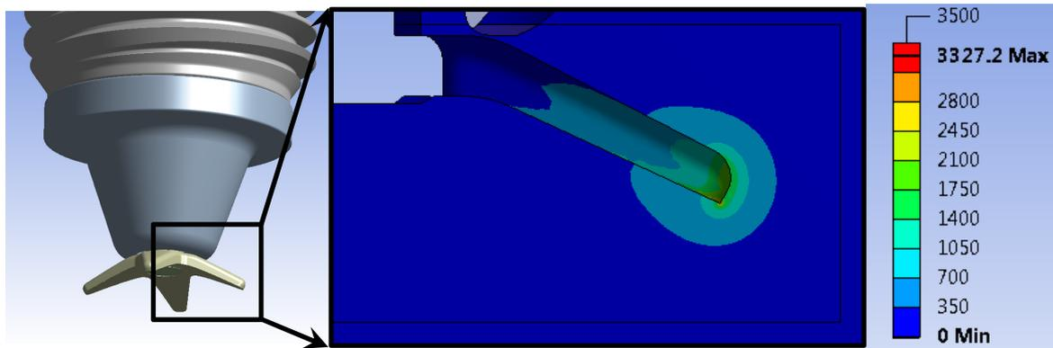
Figure 12: Electric Field Strength at Star Tip [V/m]
