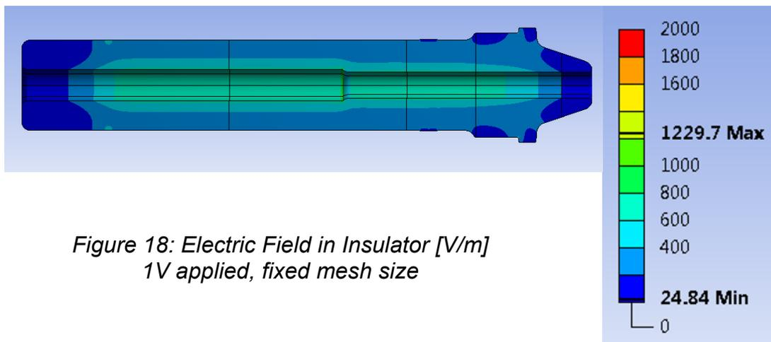
Figure 18: Electric Field in Insulator [V/m]
