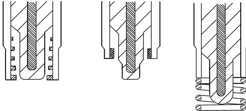
*Figure 3: Exemplary designs of a Barrier Discharge Igniter (BDI).
