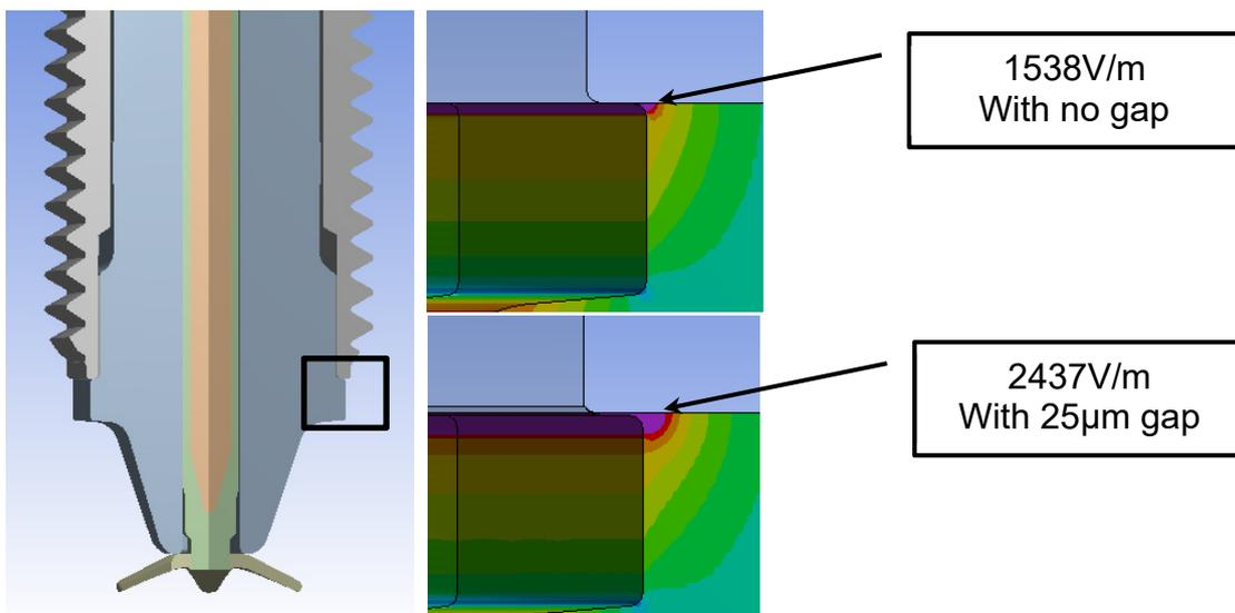
Figure 15: Electric Field at Insulator Corenose Root [V/m]
