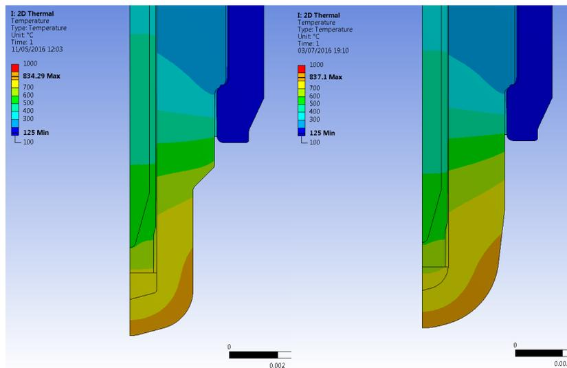
Figure 26: Thermal Performance of BDI Igniters
