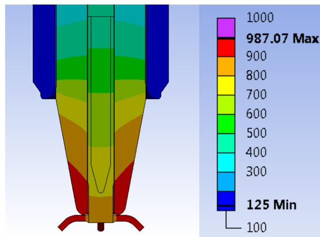
*Figure 8: Modified Central Electrode [°C]
