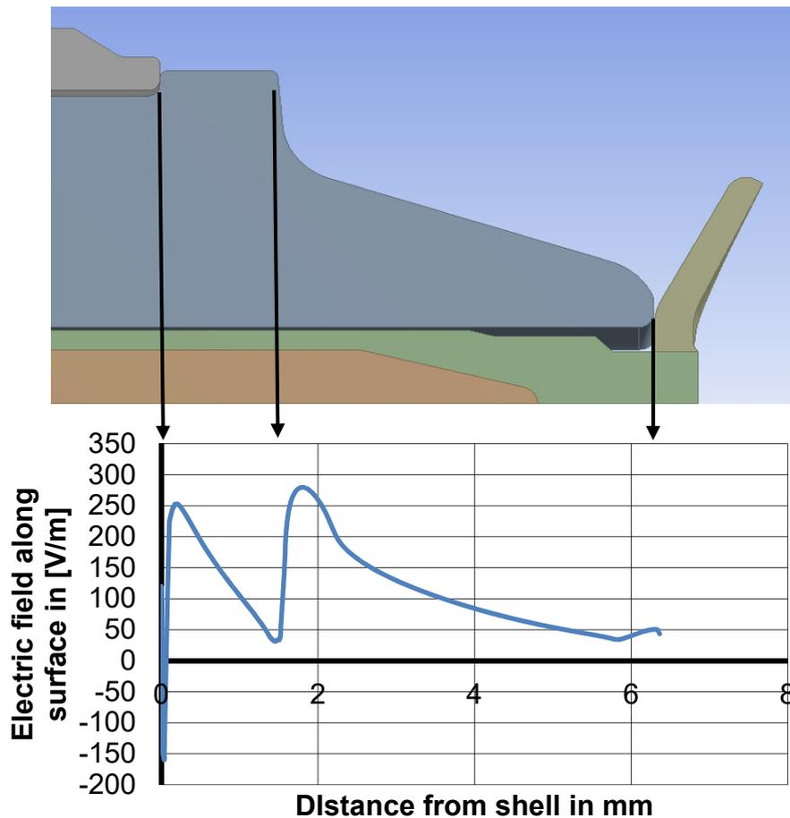
Figure 17: Electric Field over Insulator Corenose Surface [V/m]
