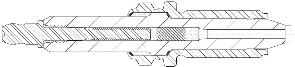
*Figure 1: Exemplary design of an arc igniter.
