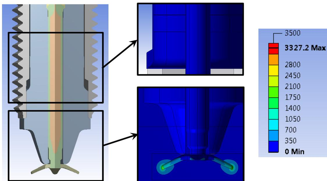
Figure 14: Electric Field Strength with Conductive Coating on Insulator [V/m]
