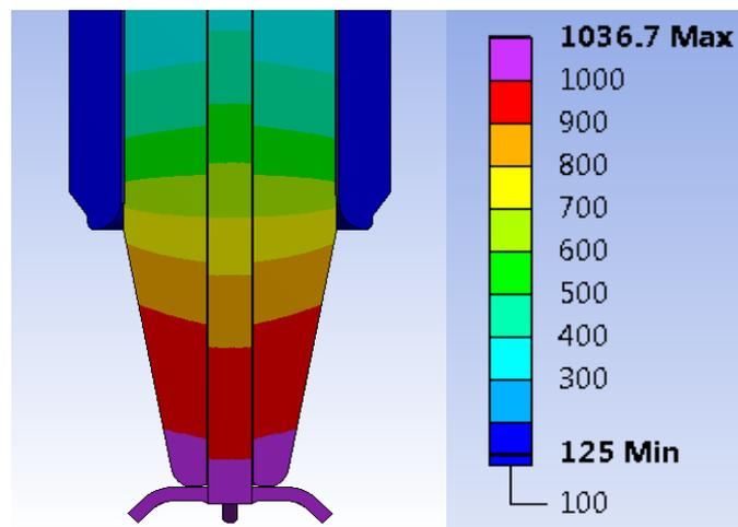
Figure 7: Early Igniter Design: Thermal Behaviour
