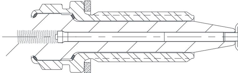
*Figure 2: Exemplary design of a streamer igniter
