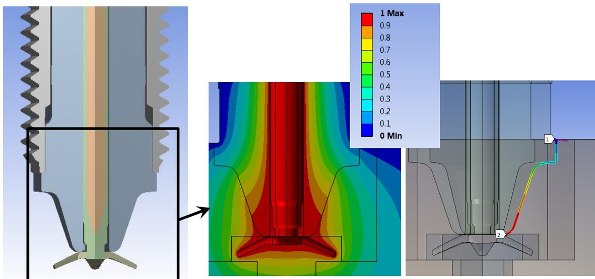
Figure 16: Voltage at Insulator Corenose Region [V]
