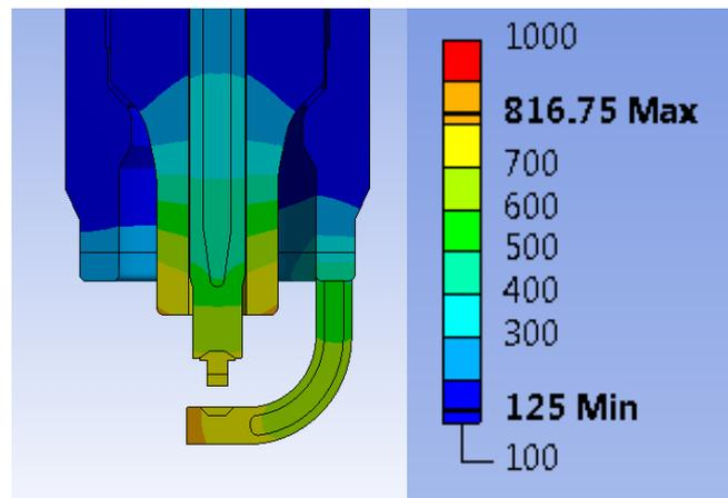
Figure 6: Example Spark Plug Thermal Field [°C]
