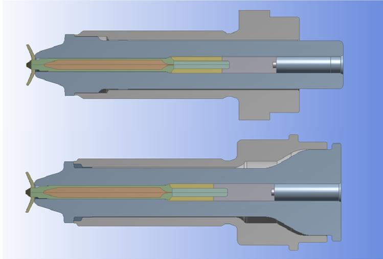
*Figure 19: m12 “Barbell” Design for Size Reduction*
