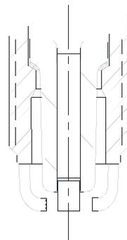
*Figure 4: Exemplary Pulse Design Igniter.
