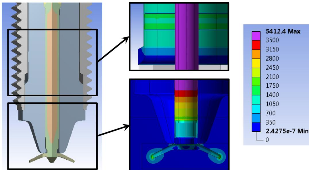
Figure 13: Electric Field Strength in Air Gaps in and around Igniter [V/m]
