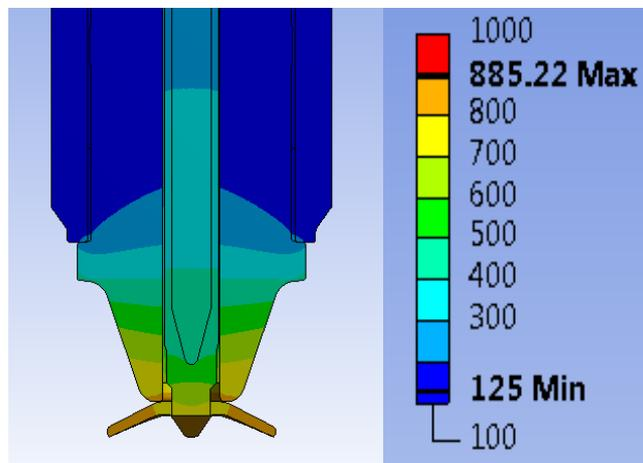
Figure 10: Reduced Corenose Length [ $^{\circ}\text{C}$ ]
