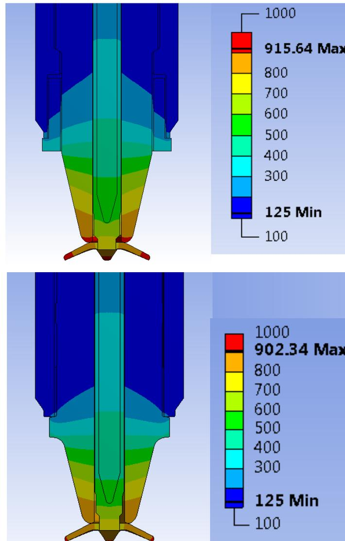
*Figure 9: Modified Lower Insulator/Shell Connection [°C]
