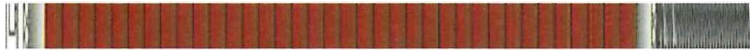
Fig. 1. One of the 5 fuel segments with a spring covered by Zr cladding at the top.
