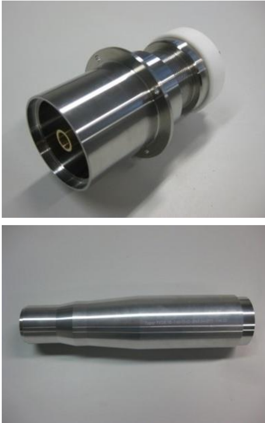
Fig. 1.1.2: Components for the TE_{28,10} mode generator: cavity with coaxial insert (left) and taper (right).
