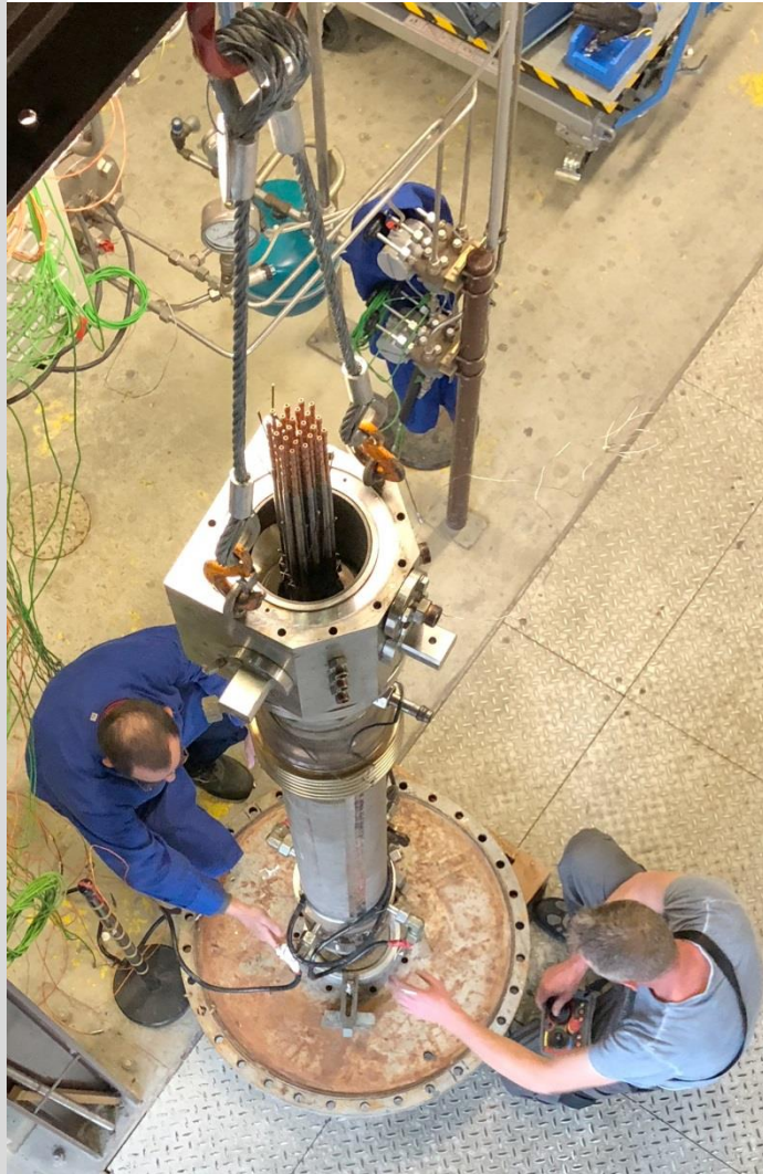
Bundle inside cooling jacket
