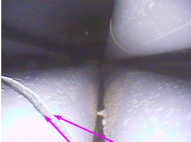
Q15: circumferential cladding cracks at hottest elevation of 950 mm
