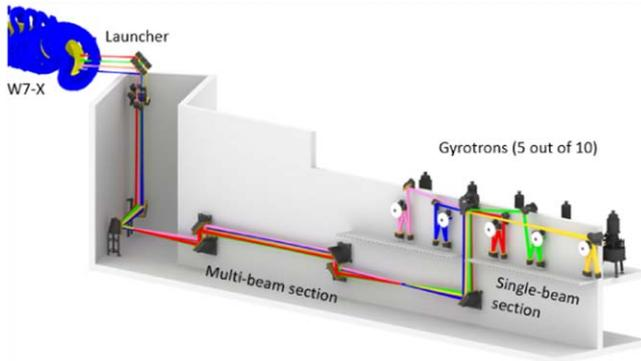
**Figure 1.** Illustration of one-half of the W7-X ECRH facility (reproduced with permission from [22]). The gyrotron beams are collected in the single-beam section and optically transmitted together over approximately 30 m in the multi-beam section, before they are divided into single beams again near the launchers. The other half of the facility (not shown) is a mirror image of the one shown.
