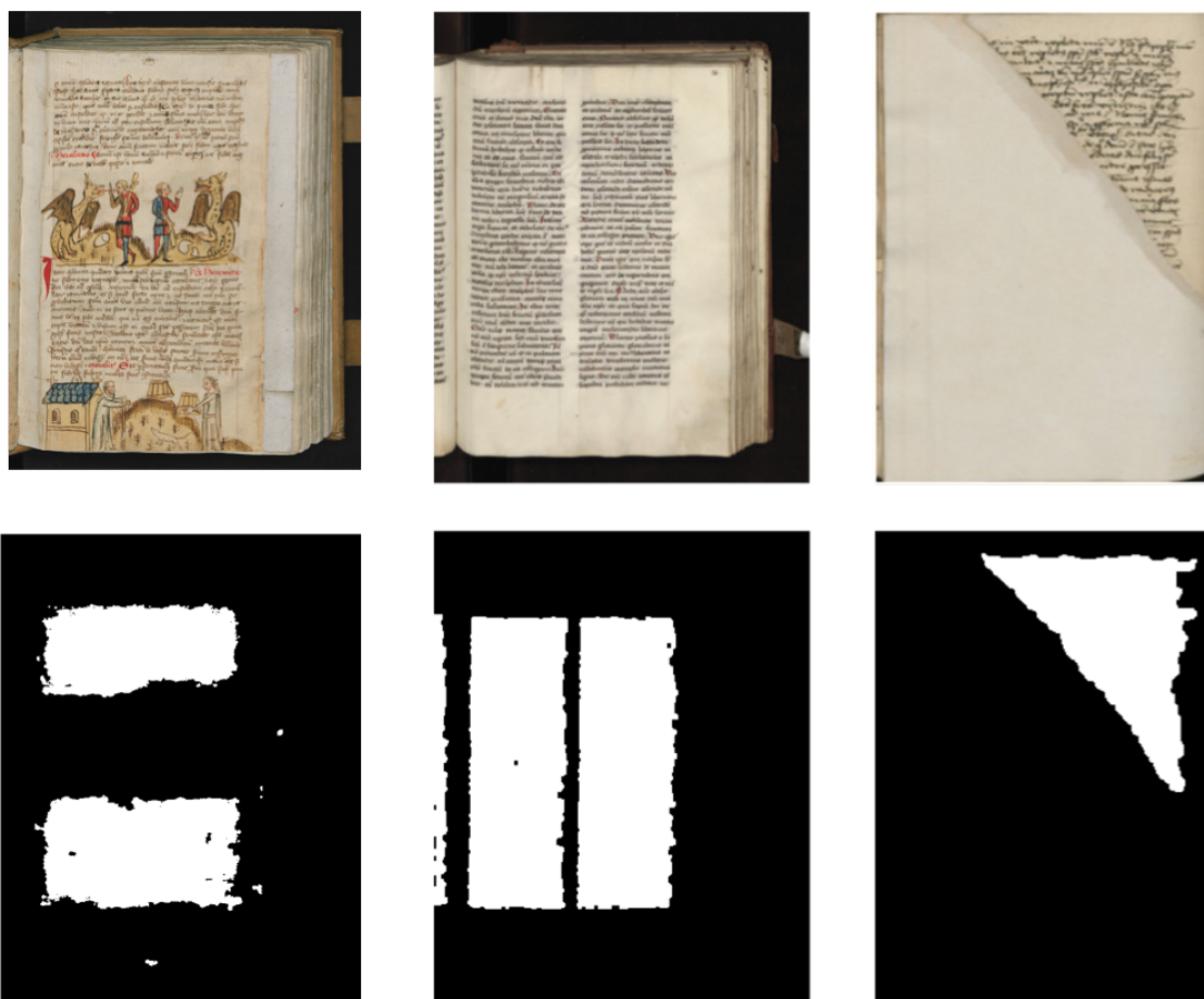
Figure 3.13 – Segmentation results for the text regions performed by pixel classification.
