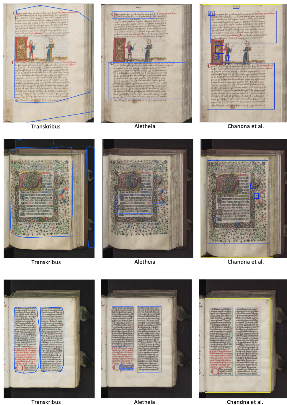
Figure 3.30 – Comparison of layout analysis approach presented by Transkribus , Aletheia , and the automatic layout approach for identification of text region presented in this thesis.
