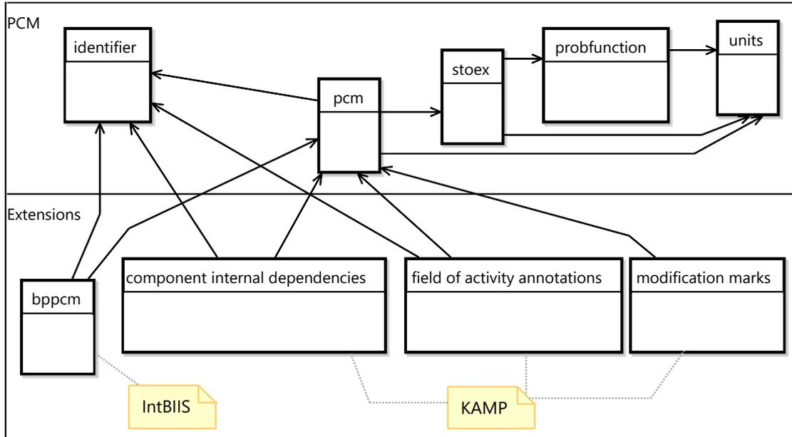
Figure 4.1: Metamodules of PCM extensions
