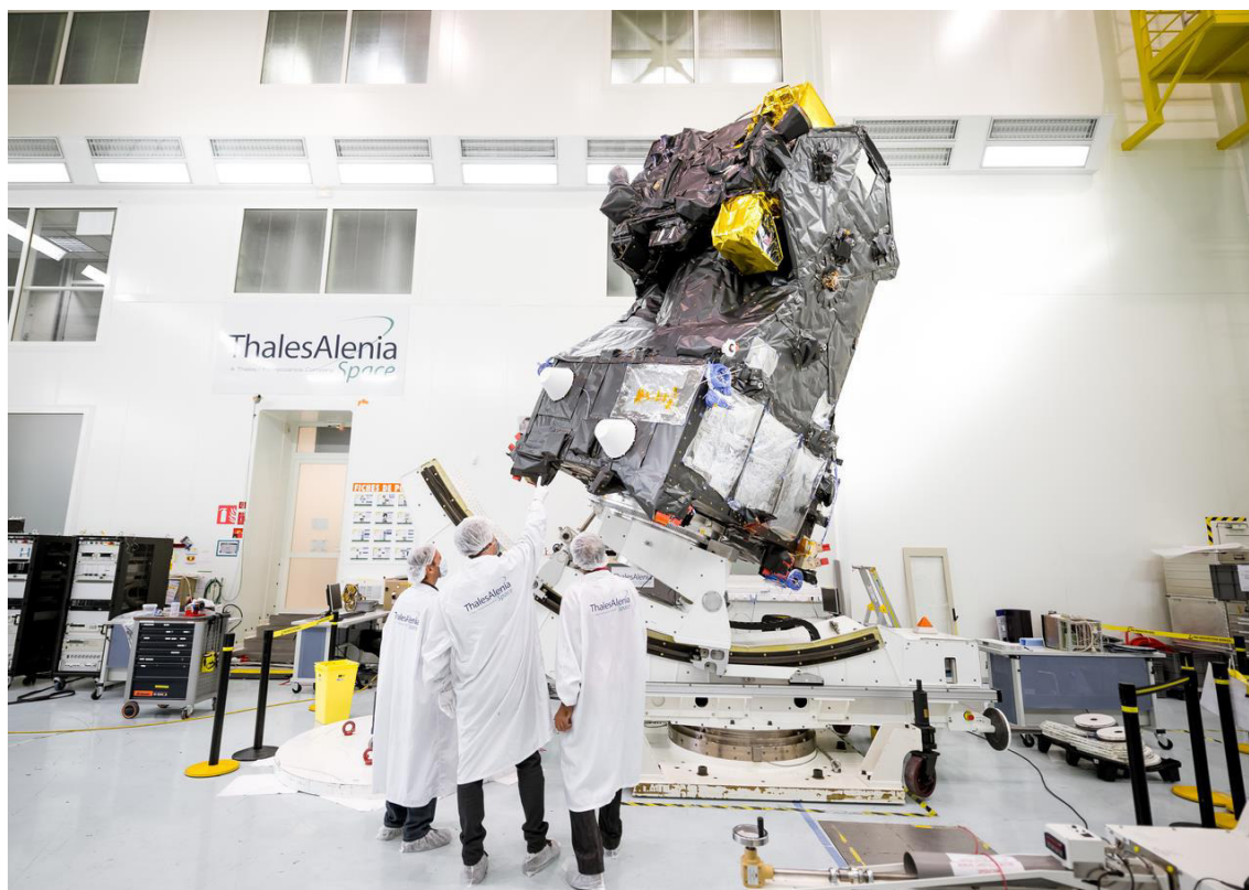
Figure 3.1: Manufacturing of the satellite ‘Trace Gas Orbiter’ at Thales Alenia Space. The satellite is covered with insulation foils for thermal control. Reprinted with permission from Thales Alenia Space [146].
