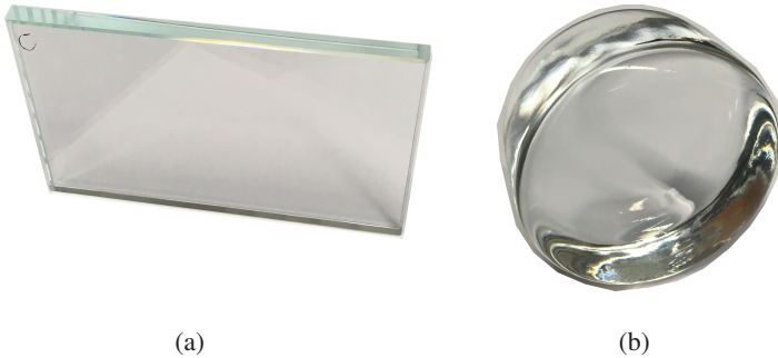
Figure 1.3: Different types of test objects: (a) a glass plate with a simple geometry is a cooperative test object; (b) a glass gob whose surface structure shows many variations is an uncooperative test object.
