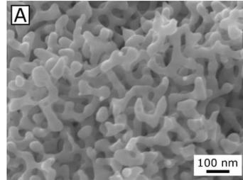
SEM image of the cross-section of a NPG sample
