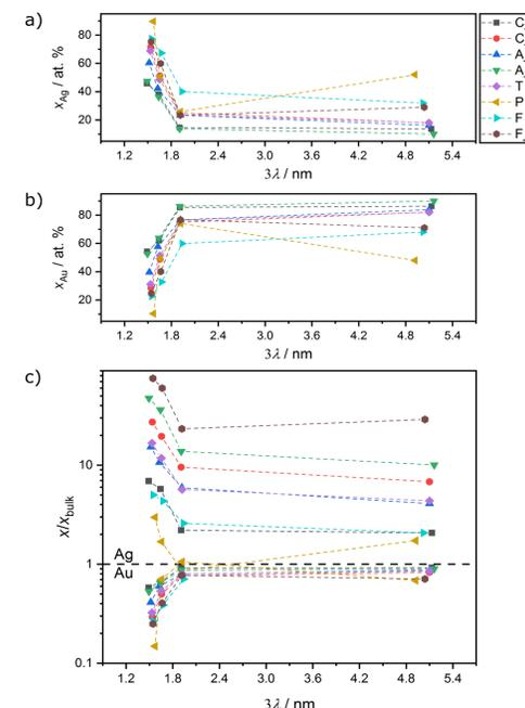
Elemental fraction of Ag (a) and Au (b) in surface-near regions of NPG and elemental fraction normalized by the bulk fraction as determined by EDX. Values > 1 indicate surface enrichment (Ag) and values < 1 indicate surface depletion (Au).
