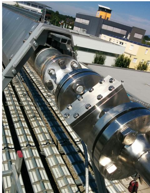
**Figure A.2: Wire Mesh Sensor installed.**
