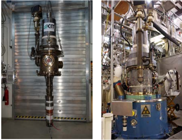
Fig. 1. The KIT 2 MW coaxial-cavity longer-pulse gyrotron (left). Gyrotron installed in the superconducting magnet (right), ready for experiments.
