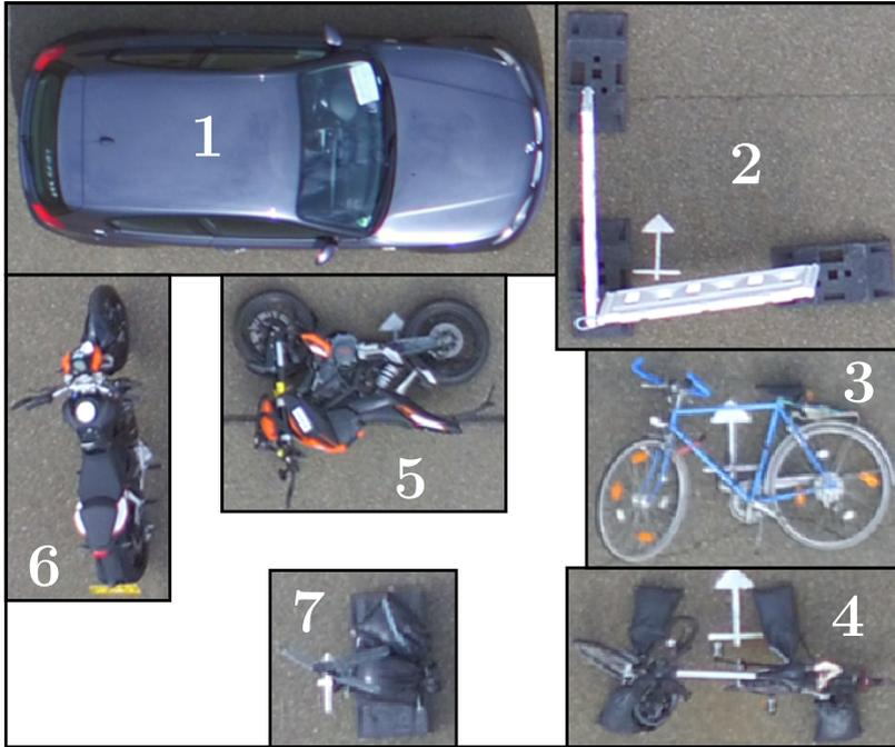
Figure 7.2: Aerial views with labels of 7 stationary targets used for classification. From 1 to 7: Car, construction barrier, lying bicycle, standing bicycle, lying motorbike, standing motorbike, and stop sign.
