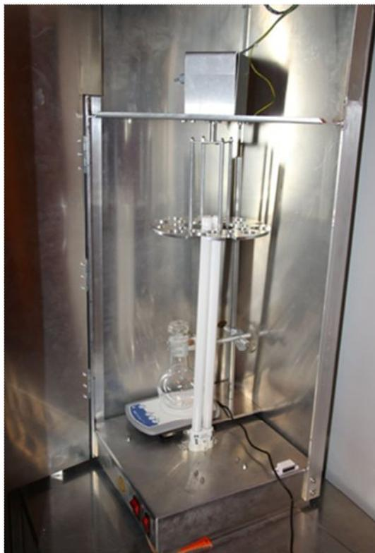
**Figure 6.1.49:** Set-up of the UV-induced formation of the SCNPs employing the Arimed B6 UV-lamp. Adapted with permission from reference [224]. Copyright (2015) American Chemical Society (ACS).<sup>224</sup>
