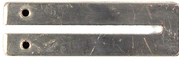
**Figure 4.2:** A U-shaped current trace with a trace width of 5 mm, a trace thickness of 2 mm and a trace gap of 2 mm.
