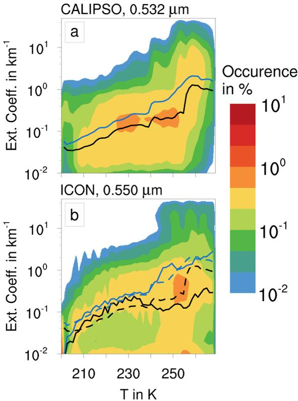
**Figure 5.4:** Two-dimensional probability distribution of the extinction coefficient with respect to temperature sampled along all tracks of CALIPSO crossing the section of the global simulation area of identical to the domain for the high-resolution simulations (Fig. 4.1) at 20 January 2016 for CALIPSO (a) and simulation *REF06* (b). Black (blue) lines indicate average (median) extinction coefficient in each temperature bin. In (b), average and median from (a) are shown as dashed lines.
