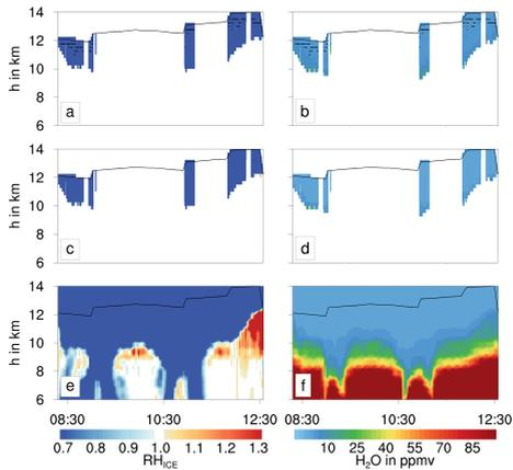
**Figure E.3:** Cross sections of relative humidity (i.e. supersaturation versus ice phase) (a) and water vapor volume mixing ratio (b) derived from GLORIA measurements during the HALO flight PGS10 on 25 January 2016. Relative humidity (c) and water vapor volume mixing ratio (d) simulated by the model and filtered for geolocations where GLORIA data are available. Full vertical cross section of the same parameters from the model simulation *REF07* (e,f). Times in UTC.
