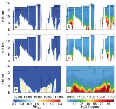
**Figure E.7:** Cross sections of relative humidity (i.e. supersaturation versus ice phase) (a) and water vapor volume mixing ratio (b) derived from GLORIA measurements during the HALO flight PGS17 on 9 March 2016. Relative humidity (c) and water vapor volume mixing ratio (d) simulated by the model and filtered for geolocations where GLORIA data are available. Full vertical cross section of the same parameters from the model simulation *REF09* (e,f). Times in UTC.
