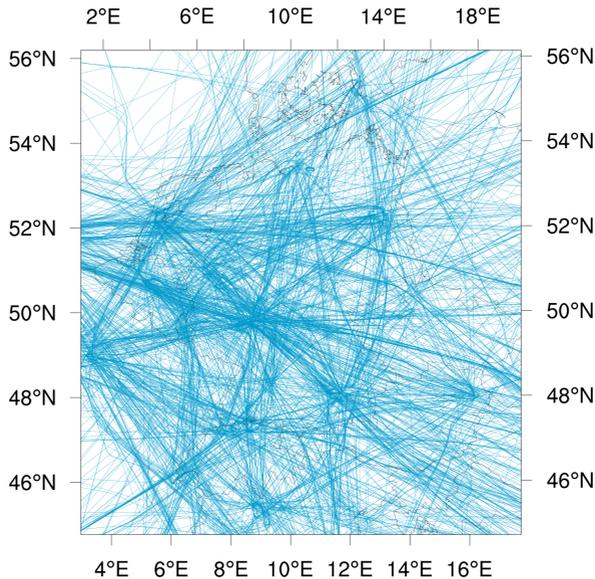
**Figure 3.2:** Flight trajectories for the simulated domain derived from ADS-B data (08 UTC - 16 UTC 3 December 2013). Each trajectory is plotted as a faint dashed line. Seemingly solid or thick lines are indicative of multiple overlaid trajectories.
