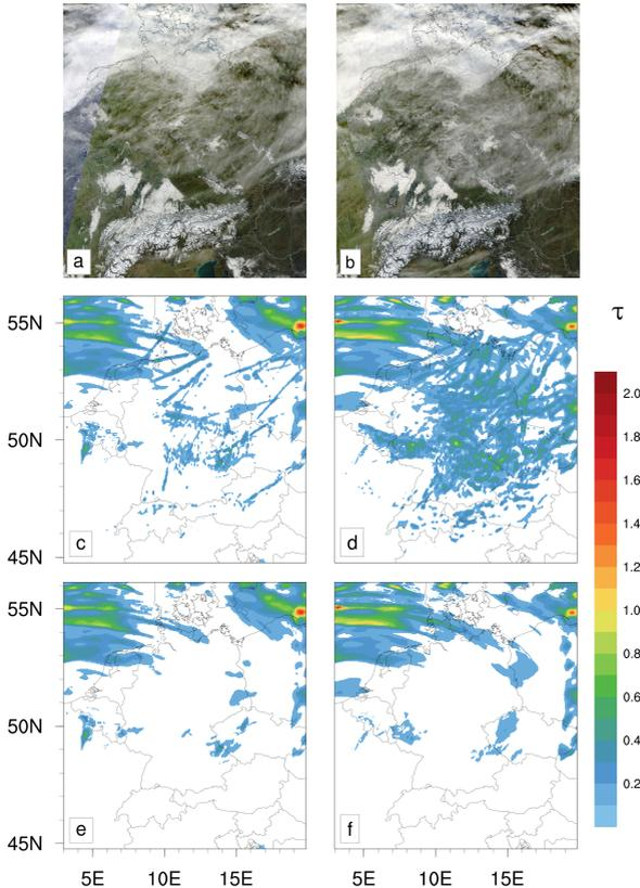
**Figure 3.10:** Top row: satellite image (MODIS True Color - Corrected Reflectance) (NASA/GSFC/ESDIS, 2018); center row: optical depth at  $1.115 \mu\text{m}$  of all ice clouds for the aviation simulation; bottom row: optical depth of all ice clouds for the reference simulation; left column: 10 UTC; right column: 12 UTC.
