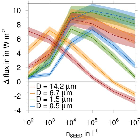
**Figure 4.22:** Changes in LW net flux at TOA (solid) and SFC (dashed) due to seeding for different combinations of  $n_{\text{SEED}}$  and  $d_{\text{SEED}}$  averaged over the entire domain and simulation time. Shaded areas represent standard errors.
