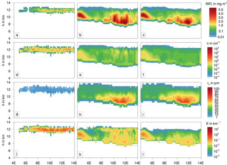
**Figure 3.7:** Vertical cross section of various contrail properties at 12 UTC along the black line in Fig. 3.4: ice water content, ice crystal number concentration, effective radius, and extinction coefficient (from top to bottom). Depicted are the simulation with aviation (left column: contrail ice class; middle column: cirrus ice class) and without aviation (right column).
