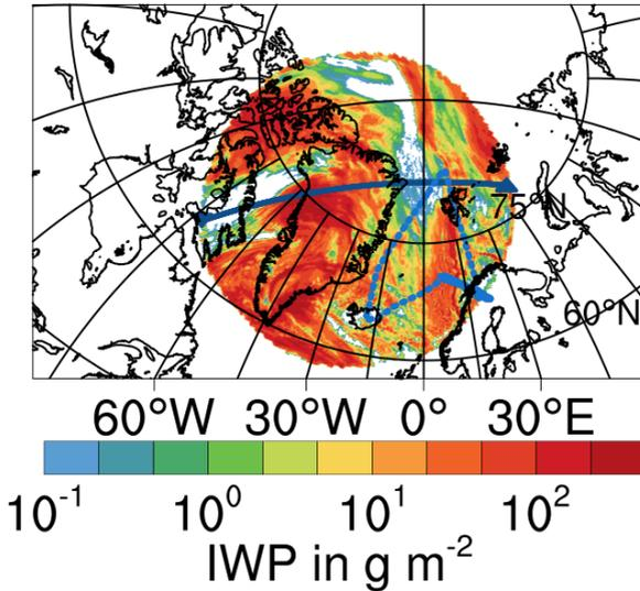
**Figure 4.3:** Simulated ice water path at 07 UTC. The dark blue line represents the CALIPSO swath crossing the domain from the location with the up- to the downward pointing triangle shown in Fig. 4.4. Light blue lines indicate flight paths (at different times of day) of HALO (dotted) and Falcon (solid).
