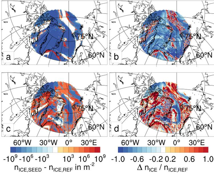
**Figure 4.14:** Difference in column integrated  $n_{ICE}$  for *SEED* and reference simulation in regions with  $T < 235$  K (top) and  $235 \text{ K} < T < 273$  K (bottom) averaged over the entire domain and simulation time. Left: absolute difference, right: relative difference.
