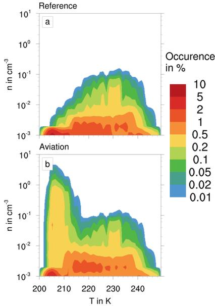
**Figure 3.8:** Relative occurrence of ice crystal number concentration versus temperature for natural cirrus, contrail and contrail cirrus at 12 UTC for the cross section along the black line in Fig. 3.4; a) reference simulation; b) aviation simulation.
