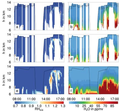
**Figure E.9:** Cross sections of relative humidity (i.e. supersaturation versus ice phase) (a) and water vapor volume mixing ratio (b) derived from GLORIA measurements during the HALO flight PGS19 on 13 March 2016. Relative humidity (c) and water vapor volume mixing ratio (d) simulated by the model and filtered for geolocations where GLORIA data are available. Full vertical cross section of the same parameters from the model simulation *REF10* (e,f). Times in UTC.
