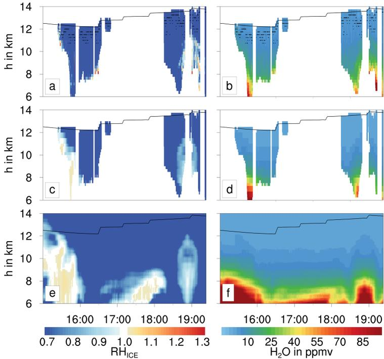
**Figure 5.6:** Cross sections of relative humidity (i.e. supersaturation versus ice phase) (a) and water vapor volume mixing ratio (b) derived from GLORIA measurements during the HALO flight PGS08 on 20 January 2016. Relative humidity (c) and water vapor volume mixing ratio (d) simulated by the model and filtered for geolocations where GLORIA data are available. Full vertical cross section of the same parameters from the model simulation REF06 (e,f). Times in UTC.
