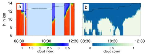
**Figure E.2:** (a) Vertical cross-section of cloud index derived from GLORIA measurements during PGS10 on 25 January 2016. Low cloud index values indicate opaque conditions due to cloud particles along the instrument's line of sight. (b) Cloud mask derived from the model simulation *REF07* at the geolocations of the measurement (0 = no cloud / 1 = cloud present). Black line in both panels: HALO flight altitude. Times in UTC.
