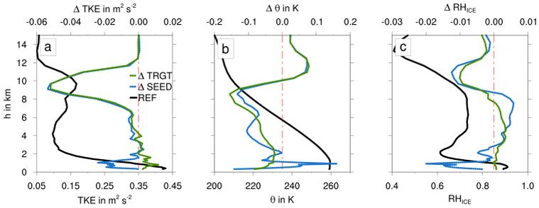
**Figure 4.18:** Changes of TKE (a), potential temperature (b) and  $RH_{ICE}$  (c) averaged over the entire domain and simulation time for reference simulation (black) and seeding strategies *SEED* (blue) and *TRGT* (green). Solid lines are absolute values, dotted lines represent differences compared to the reference simulation.
