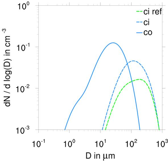
**Figure 3.1:** Ice crystal size distribution of the simulation with (blue) and without (green) aviation. For the simulation with aviation, separate ASDs of the contrail and cirrus ice class are shown (solid and dotted line). 12 UTC.
