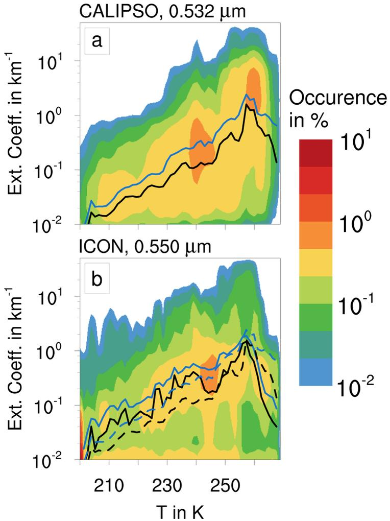
**Figure 4.5:** Two-dimensional probability distribution of the extinction coefficient with respect to temperature sampled along all tracks of CALIPSO crossing the simulation domain during the entire integration time for CALIPSO (a) and reference simulation (b). Black (blue) lines indicate average (median) extinction coefficient in each temperature bin. In (b), average and median from (a) are shown as dashed lines.
