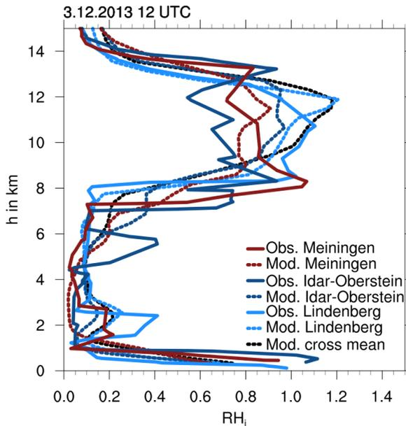
**Figure 3.6:** Radio soundings for several locations (solid lines) (UWYO, 2018) and corresponding profiles from aviation simulation (dotted lines) of relative humidity  $RH_i$ . The black dotted line are mean values along the black line in Fig. 3.4.
