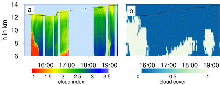
**Figure 5.5:** (a) Vertical cross-section of cloud index derived from GLORIA measurements during PGS08 on 20 January 2016. Low cloud index values indicate opaque conditions due to cloud particles along the instrument’s line of sight. (b) Cloud mask derived from the model simulation *REF06* at the geolocations of the measurement (0 = no cloud / 1 = cloud present). Black line in both panels: HALO flight altitude. Times in UTC.
