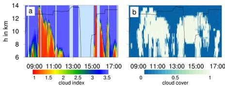
**Figure E.6:** (a) Vertical cross-section of cloud index derived from GLORIA measurements during PGS17 on 9 March 2016. Low cloud index values indicate opaque conditions due to cloud particles along the instrument's line of sight. (b) Cloud mask derived from the model simulation *REF09* at the geolocations of the measurement (0 = no cloud / 1 = cloud present). Black line in both panels: HALO flight altitude. Times in UTC.
