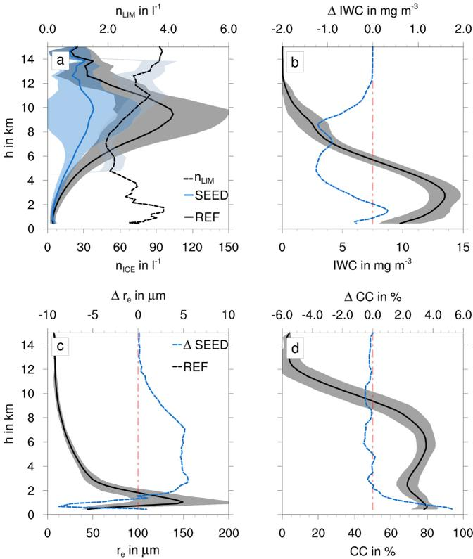
**Figure 5.9:** Comparison of ice cloud properties averaged over the entire domain and Arctic winter 2015 / 2016 for *REF* (black) and *SEED* (blue). a)  $n_{ICE}$ ; b) *IWC*; c)  $r_e$ ; d) cloud cover. Solid lines are absolute values, dotted lines represent differences compared to the reference simulation. Shaded areas indicate standard deviations. Note that in a) only absolute values are depicted, the black dotted line is  $n_{LIM}$  for *REF*.
