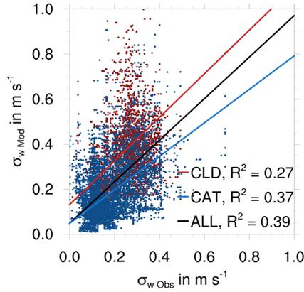
**Figure 4.10:** Comparison of  $\sigma_w$  for simulated ( $f_w = 0.3$  in Eq.2.37) and observed vertical velocity. The lines represent linear regression of all points (black), cloud-free regions (blue), and in-cloud regions (red). For details, see text.
