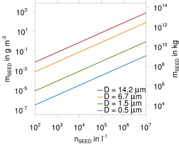
**Figure 4.23:** Mass of seeding aerosol for different combinations of  $n_{\text{SEED}}$  and  $d_{\text{SEED}}$ . Left axis represents column-integrated mass per  $\text{m}^2$ , right axis represents total aerosol mass for the entire Arctic region (i. e. north of  $60^\circ\text{N}$ ).
