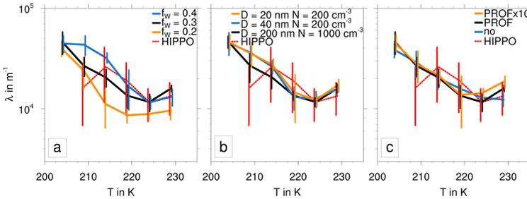
**Figure 4.11:** Temperature dependence of the slope parameter  $\lambda$  (Eq. 4.2) for HIPPO measurements (red, dotted) and simulations (solid) with different values for  $f_w$  (a), sulphate aerosol properties (b), and dust concentrations (c). The vertical bars denote the standard deviation.
