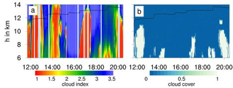
**Figure E.4:** (a) Vertical cross-section of cloud index derived from GLORIA measurements during PGS14 on 26 February 2016. Low cloud index values indicate opaque conditions due to cloud particles along the instrument's line of sight. (b) Cloud mask derived from the model simulation *REF08* at the geolocations of the measurement (0 = no cloud / 1 = cloud present). Black line in both panels: HALO flight altitude. Times in UTC.
