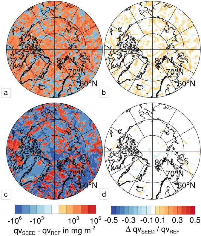
**Figure 5.11:** Difference in column integrated water vapor content between *SEED* and *REF* in regions with  $T < 235$  K (top) and  $235\text{ K} < T < 273$  K (bottom) averaged over the entire domain and Arctic winter 2015 / 2016. Left: absolute difference, right: relative difference.
