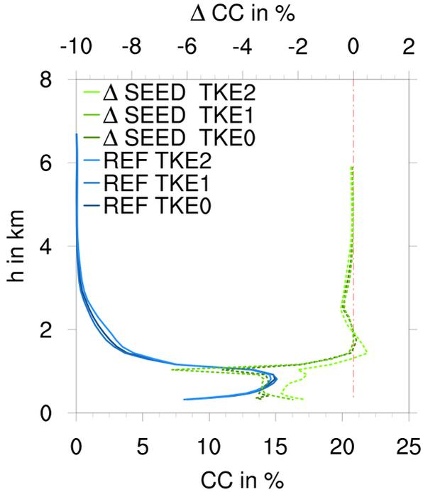
**Figure D.2:** Comparison of liquid (mixed-phase) cloud cover for different values of  $f_w$  averaged over the entire domain and simulation time for reference simulations (blue) and simulations with  $n_{\text{SEED}} = 10^3 \text{ l}^{-1}$  and  $d_{\text{SEED}} = 6.7 \text{ }\mu\text{m}$ . Solid lines are absolute values, dotted lines represent differences compared to the reference simulation.
