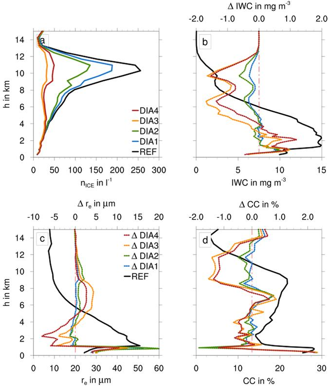
**Figure 4.19:** Comparison of ice cloud properties averaged over the entire domain and simulation time for reference simulation (black) and simulations with  $n_{SEED} = 10^3\ l^{-1}$  and various  $d_{SEED}$  (colors). a)  $n_{ICE}$ ; b)  $IWC$ ; c)  $r_e$ ; d) cloud cover. Solid lines are absolute values, dotted lines represent differences compared to the reference simulation. Note that in a) only absolute values are depicted.
