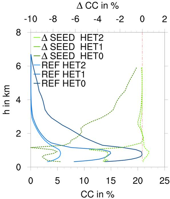
**Figure D.6:** Comparison of liquid (mixed-phase) cloud cover for different dust aerosol concentrations averaged over the entire domain and simulation time for reference simulations (blue) and simulations with  $n_{\text{SEED}} = 10^3 \text{ l}^{-1}$  and  $d_{\text{SEED}} = 6.7 \mu\text{m}$ . Solid lines are absolute values, dotted lines represent differences compared to the reference simulation.
