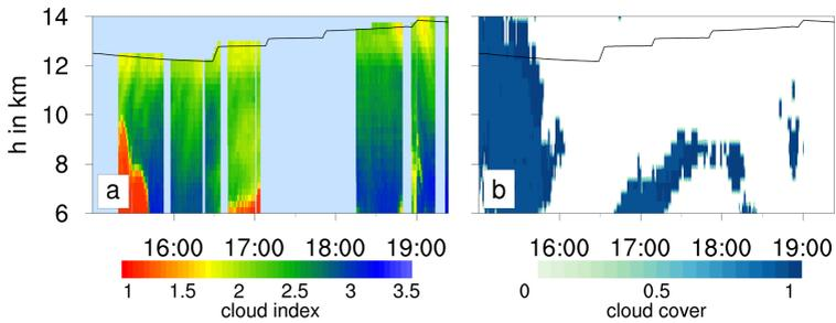
**Figure 4.6:** (a) Vertical cross-section of cloud index derived from GLORIA measurements during PGS08 on 20 January 2016. Low cloud index values indicate opaque conditions due to cloud particles along the instrument’s line of sight. (b) Cloud mask derived from the model simulation at the geolocations of the measurement (0 = no cloud / 1 = cloud present). Black line in both panels: HALO flight altitude. Times in UTC.
