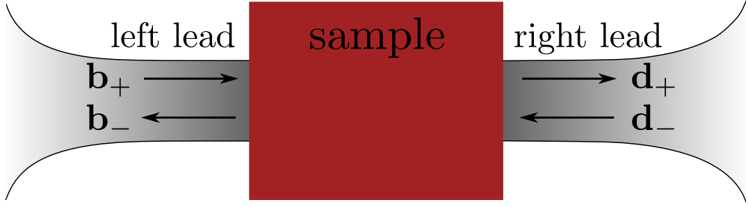
Figure 2.4: Geometry of a mesoscopic system considered for the derivation of Landauer formula. The system consists of a left and a right lead where the amplitudes of the wave functions are given by \mathbf{b}_+ , \mathbf{b}_- for the left and \mathbf{d}_+ , \mathbf{d}_- for the right lead. These four states scatter at the sample.
