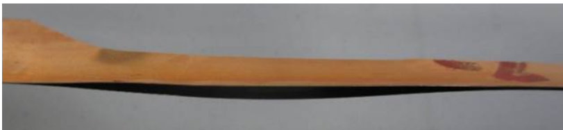
Figure A.5: Delamination in a Fujikura tape that appeared after punching.
