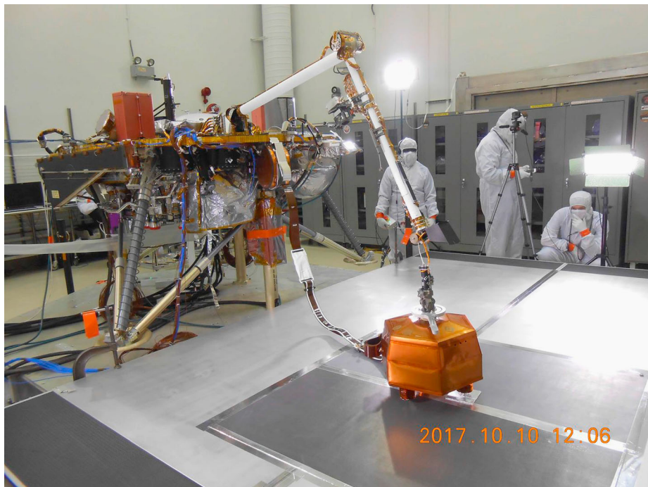
Fig. 12 The Sensor Assembly being deployed on the ground during DST#3 (Deployment System Test). Two segments of the tether (TSA-1, part of TSA-), the Tether Storage Box, Field Joint and part of the Load Shunt Assembly are also visible
